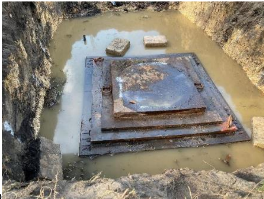
Figure 6-36 (a) picture of 28 in by 28 in steel plate before test; (b) picture of 28 in by 28 in steel plate after test; (c) picture of 48 in by 48 in steel plate after test with settlements at each location
