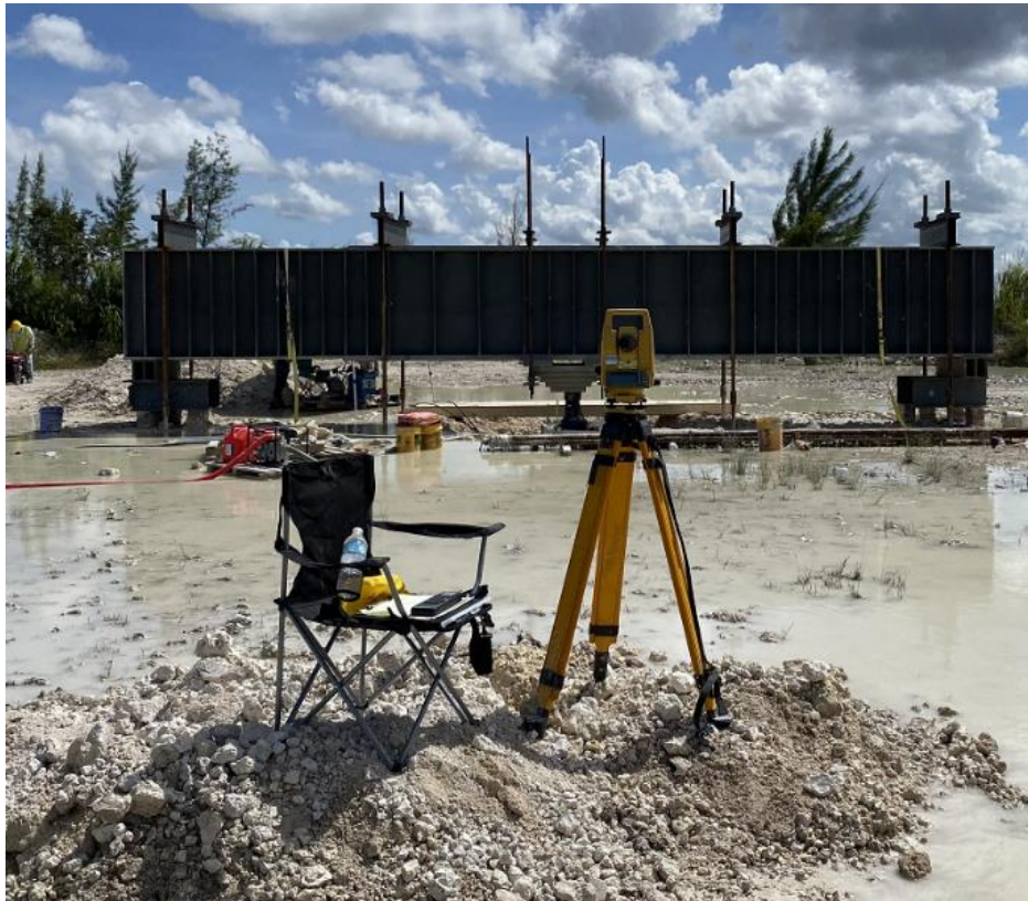
Figure 5-26 (a) locations of tape measures and measuring frame; (b) total station
