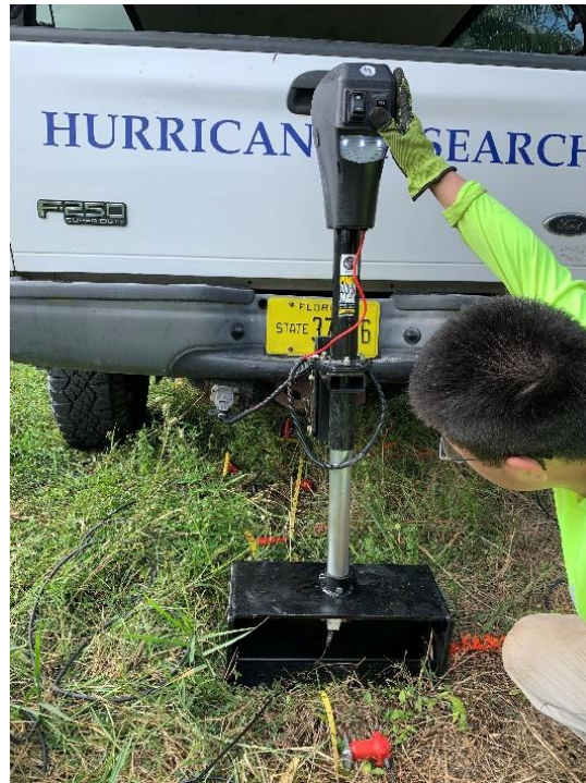
Figure 4-14 The shear-beam pressed by the hydraulic jack
