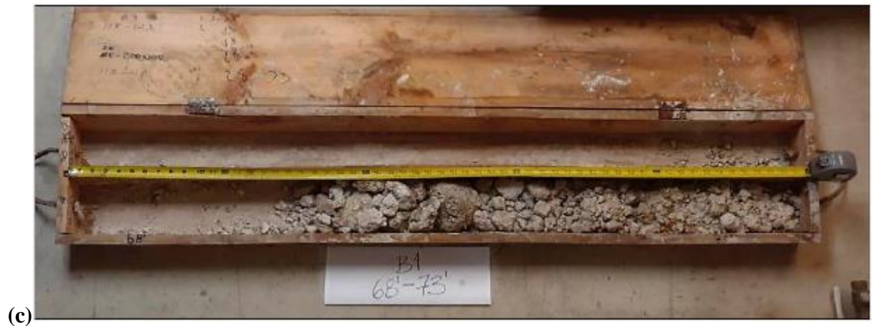
Figure B-7 Pictures of rock cores for B-1. (a): 3 ft – 13 ft; (b): 33 ft – 43 ft; (c): 68 ft – 73 ft
