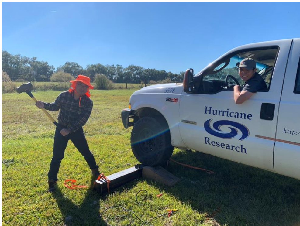
Figure 4-27 The shear-beam pressed by the vehicle wheel
