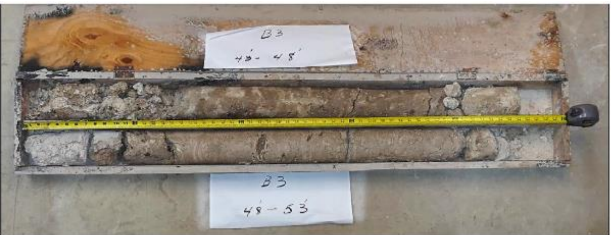
Figure B-9 Pictures of rock cores for B-3. (a): 3 ft – 13 ft; (b): 33 ft – 43 ft; (c): 43 ft – 53 ft
