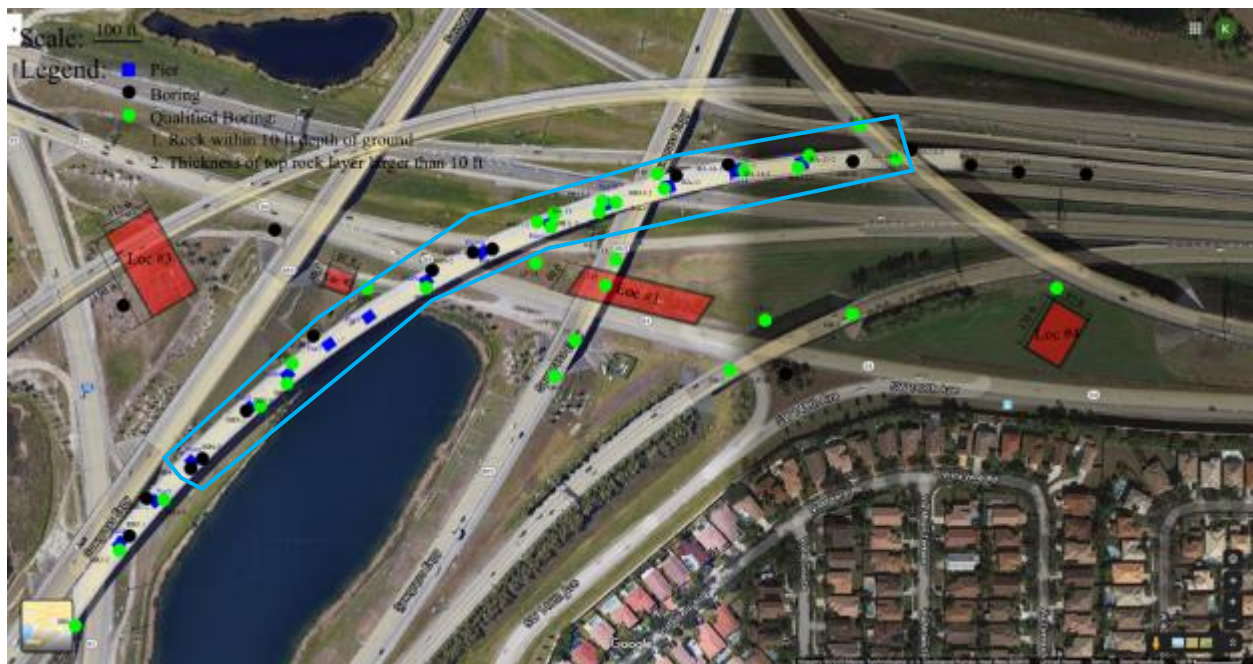
Figure 6-39 Boring and pier locations at the SR-84 site (I-75 express lanes segment E)
