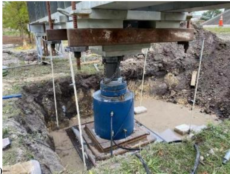
Figure 6-32 Measuring system. (a): from a ground surface view; (b): bricks used to make the scaffolding base plate fully contact with the footing (5 ft by 6 ft steel plate)
