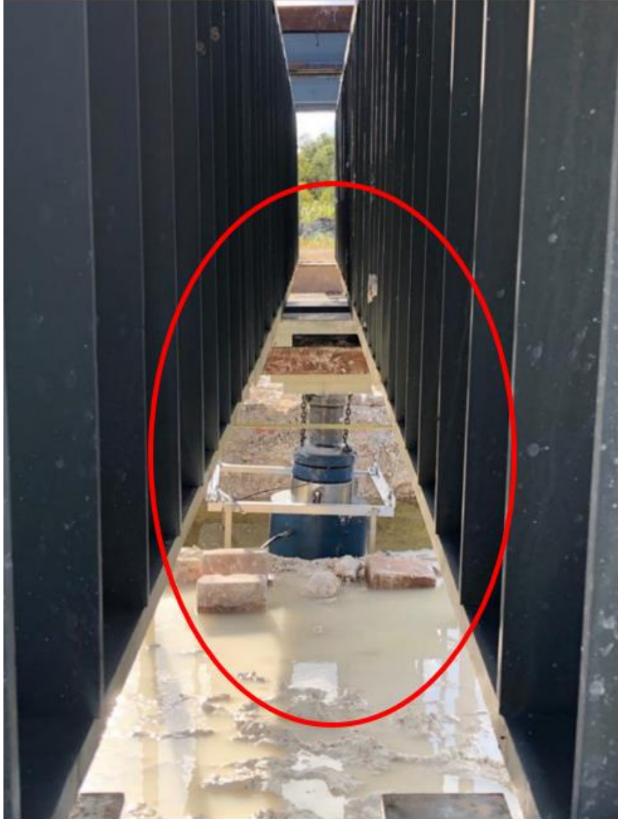
Figure 5-29 Inclination of the loading jack and load cell
