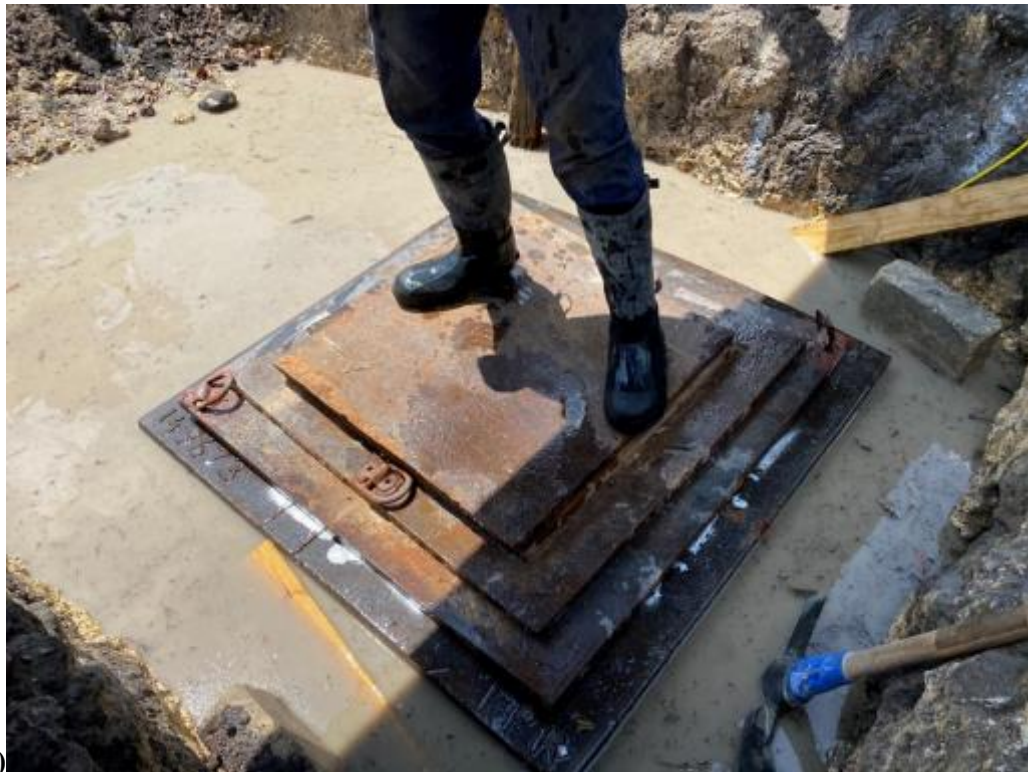
Figure 6-31 Eight steel plates representing the footing. (a): lower 4 steel plates, top to down: 4 ft by 4 ft, 4 ft by 4 ft, 4 ft by 6 ft and 5 ft by 6 ft; (b): upper 4 steel plates, top to bottom: 28 in by 28 in, 28 in by 28 in, 36 in by 36 in and 42 in by 42 in
