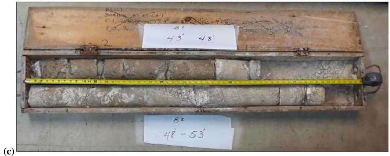
Figure B-8 Pictures of rock cores for B-2. (a): 3 ft – 13 ft; (b): 33 ft – 43 ft; (c): 43 ft – 53 ft
