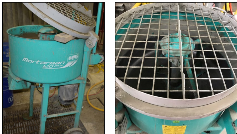
Figure F.5: Mortar Mixer used to Mix CLSM Grout: Side View (left), Top View (right).
