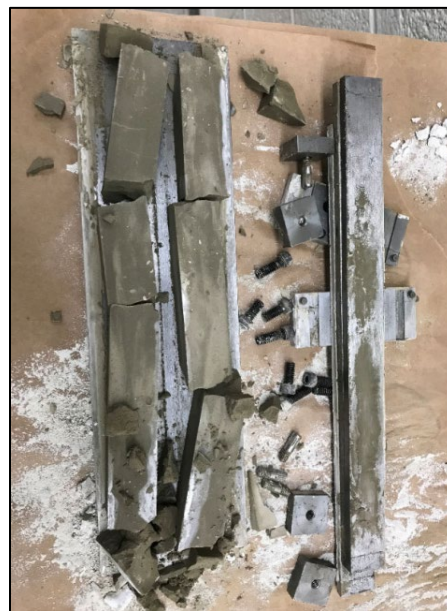
Figure F.35: Broken Shrinkage Samples Prepared from CLSM Mix C.
