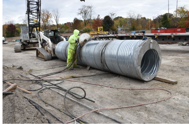
(b) Cutting of culvert specimens
