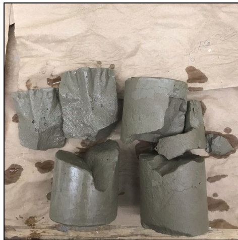
Figure F.37: Broken Water Absorption Sample (Mix C).
