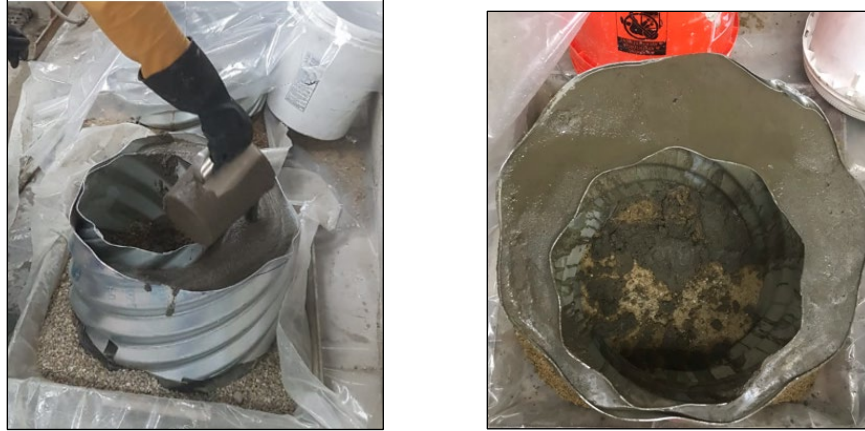
Figure F.21: Filling Annulus Voids of a Type I Culvert with CLSM Grout (Mix A-5): Pouring the Grout ( left ), Culvert Specimen with Fully Grouted Annulus ( right ).
