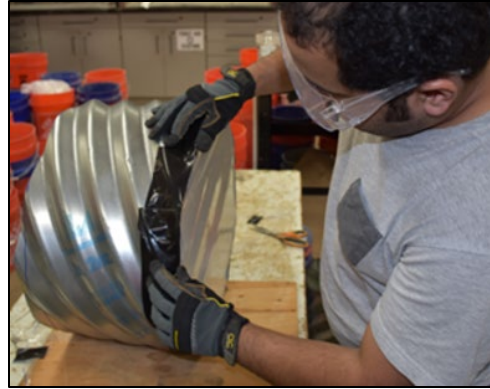
(b) Wrapping the pipe end with plastic.
