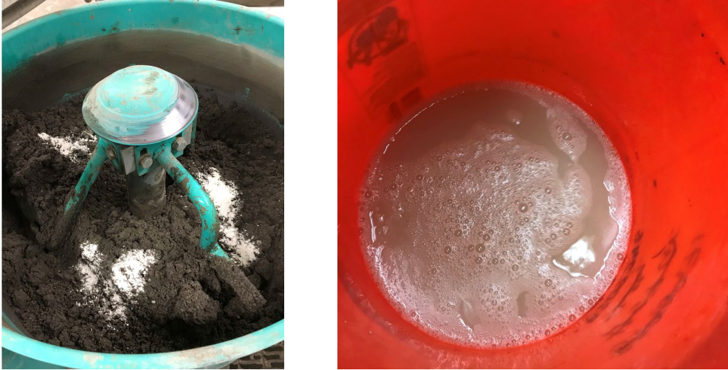
Figure F.3: Mixing Fill Flow: Adding Powder Directly to the Mix (left), Mixing Fill Flow with Water Prior to Adding it to the Mix (right).
