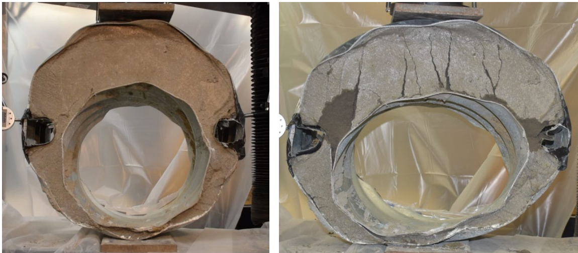
Figure F.47: Sliplined Culvert with Voids at the Springline, Before ( left ) and After ( right ) the Parallel-Plate Loading Test.
