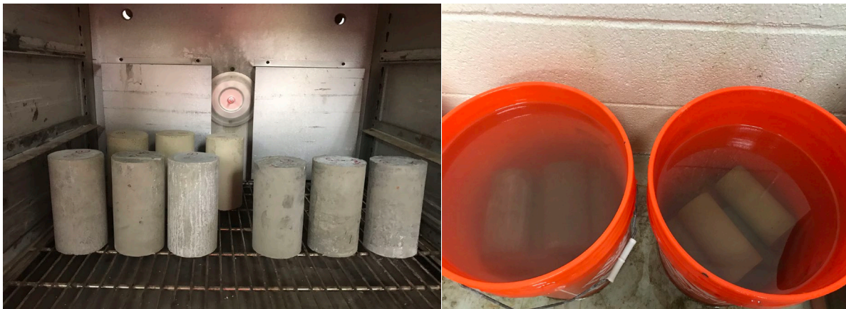
Figure F.16: Water Absorption Test of CLSM Specimens: CLSM Specimens in the Oven ( left ), CLSM samples Submerged in Water ( right ).
