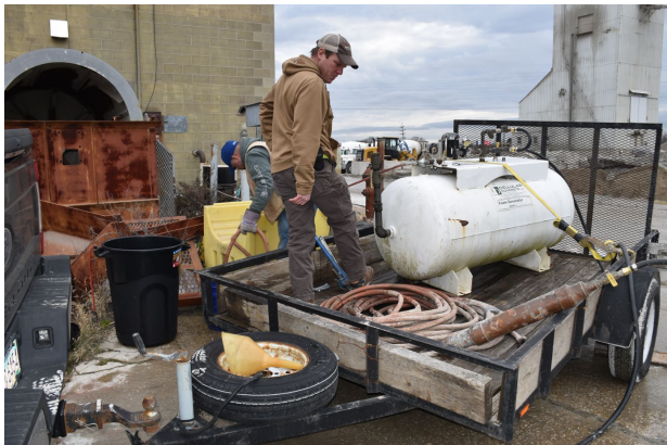
(c) Creating Foam with a Foam Generator
