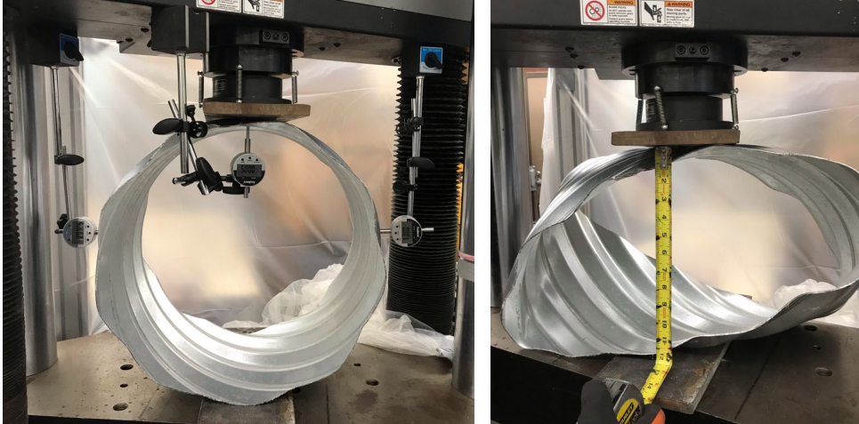
Figure F.41: Parallel-Plate Loading Tests: Liner Pipe Before ( left ) and After Loading ( right )
