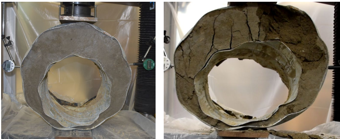
Figure F.42: Sliplined Culvert with CLSM grout Mix A Before ( left ) and After ( right ) the Parallel-Plate Loading Test.
