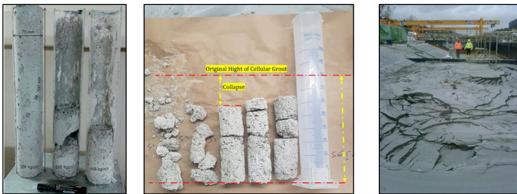
Figure 6: Instability of Ultra-Low Cellular Grout: (a) Lab-prepared Grout from Jones et al. 2016 (left), (b) Lab-prepared Cellular Grout C10 (center), and On-site Instability for Grout Reported by Jones et al. 2016 (right).
