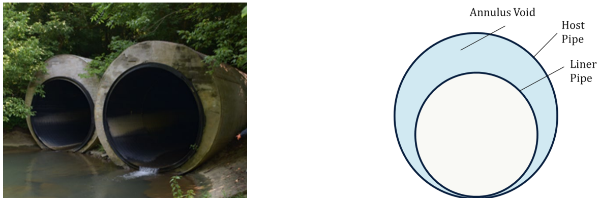
Figure 1: Image ( Left ) and Schematic Diagram ( Right ) of Typical Sliplined Culverts.
