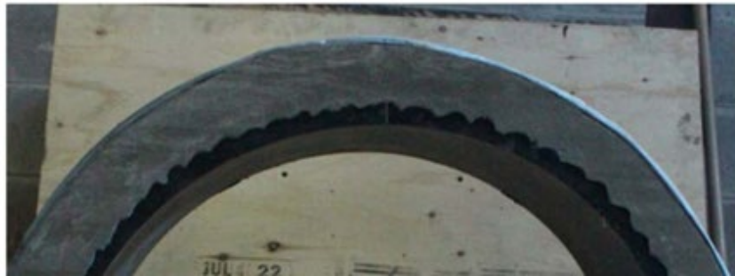
(b) No apparent shrinkage in the low-strength grout specimen
