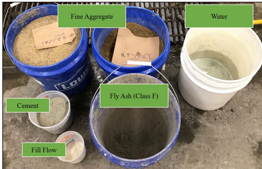
Figure F.4: Measured Mixture Components Needed to Produce One Cubic Foot of CLSM Mix.
