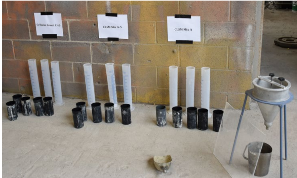
Figure G.2: Test Station for Tests on Fresh and Hardened Properties of the Cellular Grout and CLSM Grouts.
