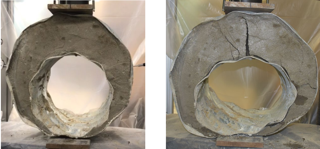
Figure F.43: Sliplined Culvert with CLSM grout Mix A-5 Before ( left ) and After ( right ) the Parallel-Plate Loading Test.
