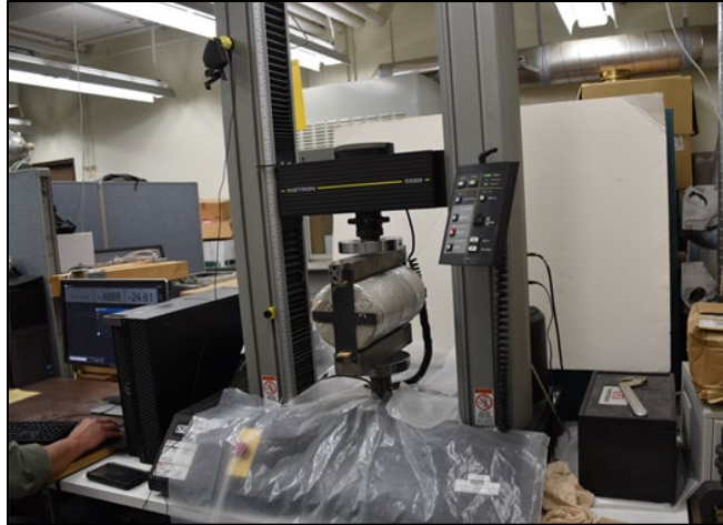
Figure E.14: Setup for Split Tensile Test.
