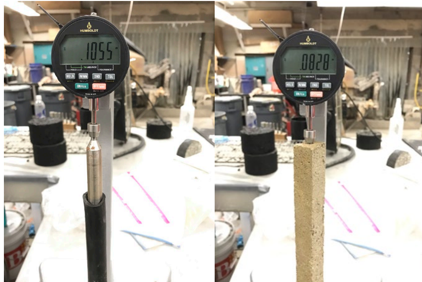
Figure F.15: Determination of the Change in Length of a CLSM Sample: Measuring an Invar Reference Bar in the Length Comparator ( left ), Length Comparator with a Shrinkage Sample of CLSM ( right ).
