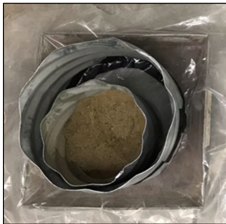
(c) Prepared host and liner pipe.
