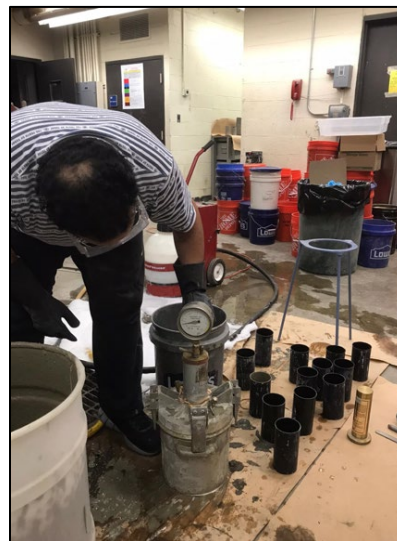
(b) Conducting Air Content Test.
