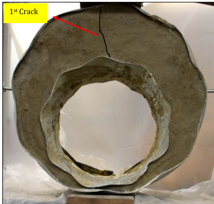
Figure E.57: First Crack Occurred in CLSM Mix A Grout at 1,300 lbf.
