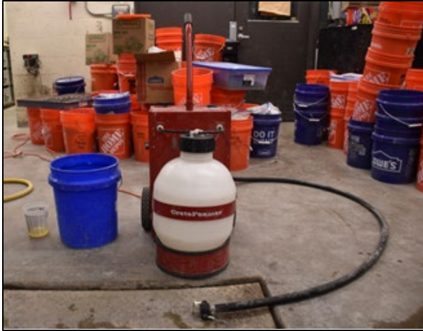
(a) Setup for Foam Generator
