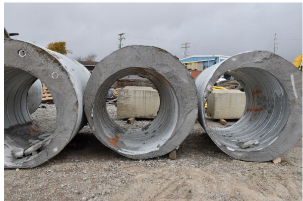
Figure 13: Cut Surfaces of Test Specimens for Culvert Grouted with CLSM (left) and Culvert Grouted with Cellular Grout (right).
