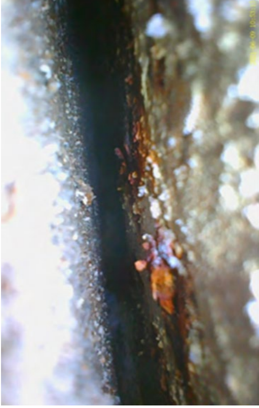
(c) Delamination (left: at the liner pipe; right: at the host pipe)
