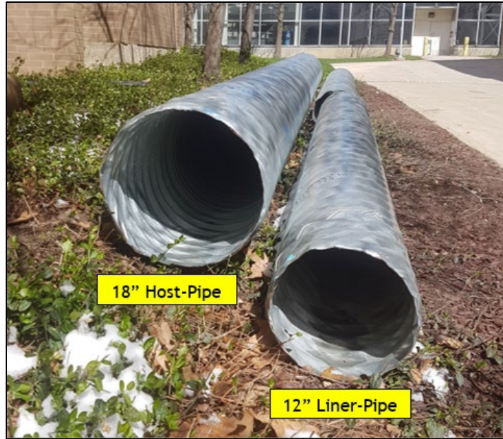
Figure E.18: Galvanized Corrugated Steel Pipes used as a Host Pipe and a Liner Pipe.
