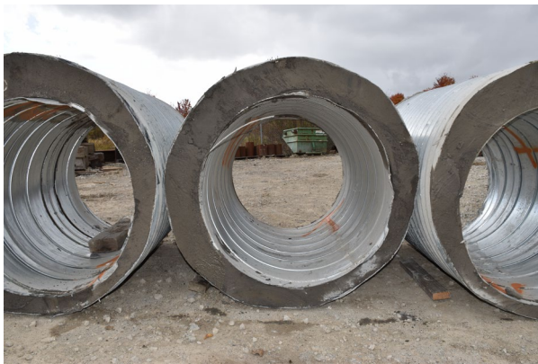
Figure 13: Cut Surfaces of Test Specimens for Culvert Grouted with CLSM (left) and Culvert Grouted with Cellular Grout (right).
