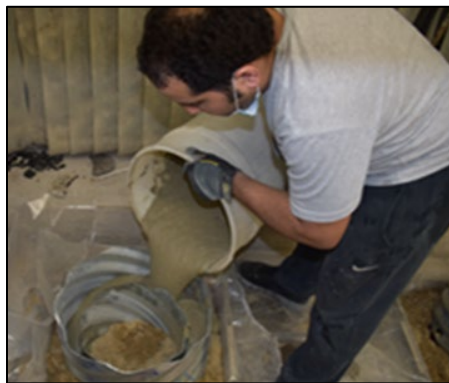
Figure E.21: Filling Annulus Voids with C40 Cellular Grout: Pouring the Grout ( left ) and Smoothing the Grout at the Surface ( right ).
