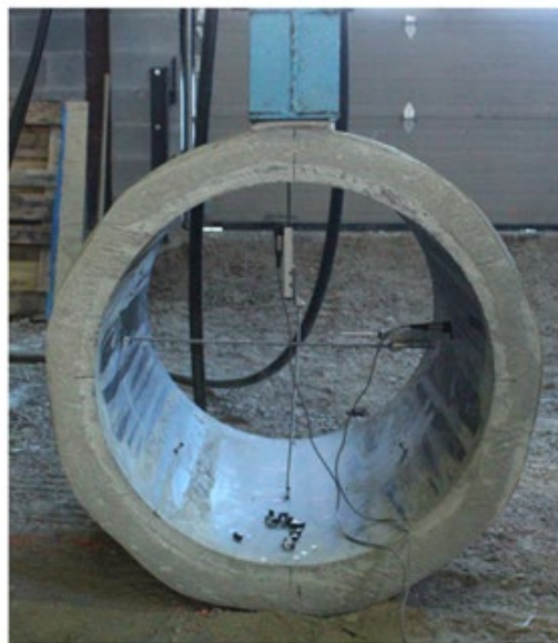
Figure A.36: Two-point loading setup showing the low-strength grout specimen with the liner (Smith et al. 2015).
