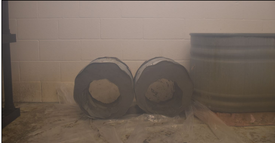
Figure E.25: Sliplined Culvert Samples in the Curing Room.
