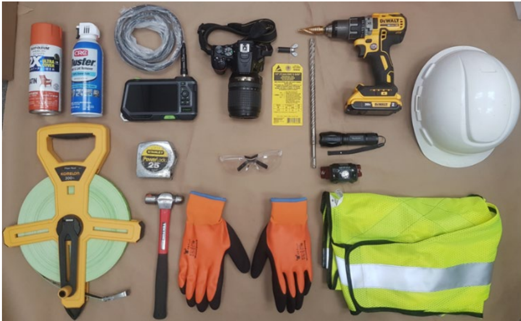
Figure C.1: Inspection Tools and Safety Gear for Conducting Sounding Tests.
