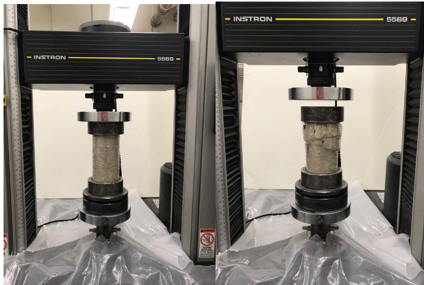
Figure F.13: Unconfined Compressive Strength Test: Setup with Specimen Loaded into Test Frame ( left ), Test Specimen that Failed when Loaded ( right ).
