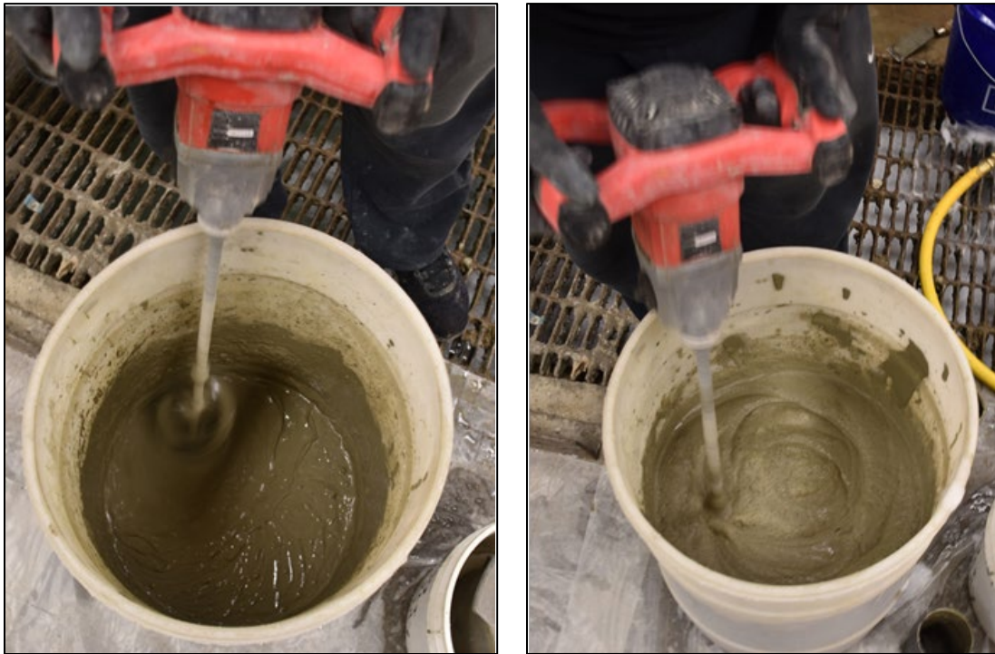
Figure E.4: Addition of Foam to a Cement Mixture: Before ( left ) and After ( right ) Addition of Foam.
