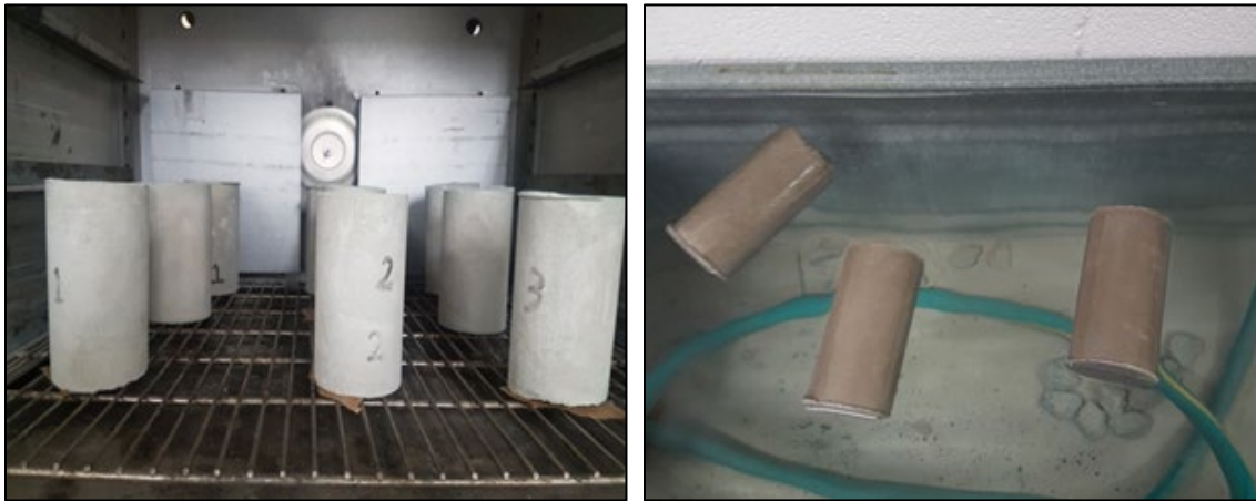
(a) Oven-drying of Cylinder Specimens. (b) Specimens Immersed in Water.
