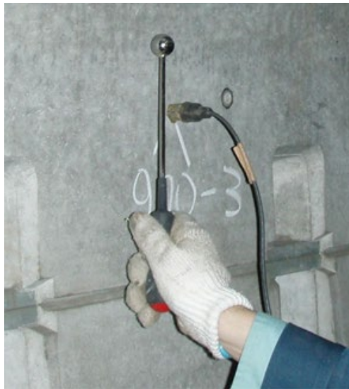
Figure A.72: Excitation using a 1-inch (25-mm) impact hammer near the accelerometer (Aggelis et al. 2008).
