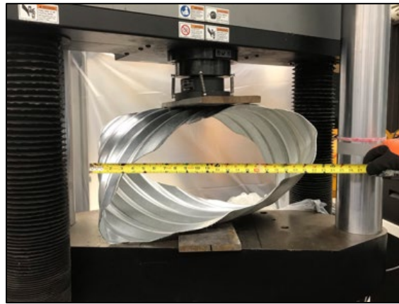
(b) Liner Pipe after Loading.
