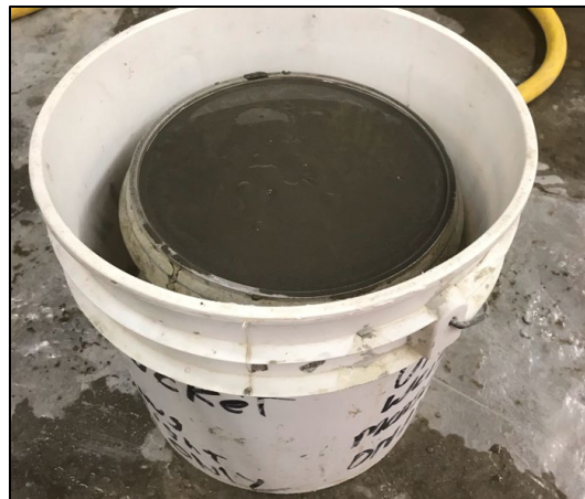
Figure F.10: Density Test for Freshly Mixed CLSM.
