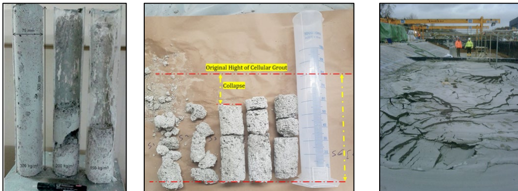
Figure E.39: Instability of Ultra-Low Cellular Grout: (a) Lab-prepared Grout from Jones et al. 2016 (left), (b) Lab-prepared Cellular Grout C10 (center), (c) and On-site Instability for Grout Reported by Jones et al. 2016 (right).
