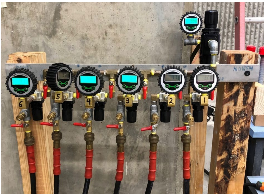
Figure 6-1. Matjack system manifold with six bays.
