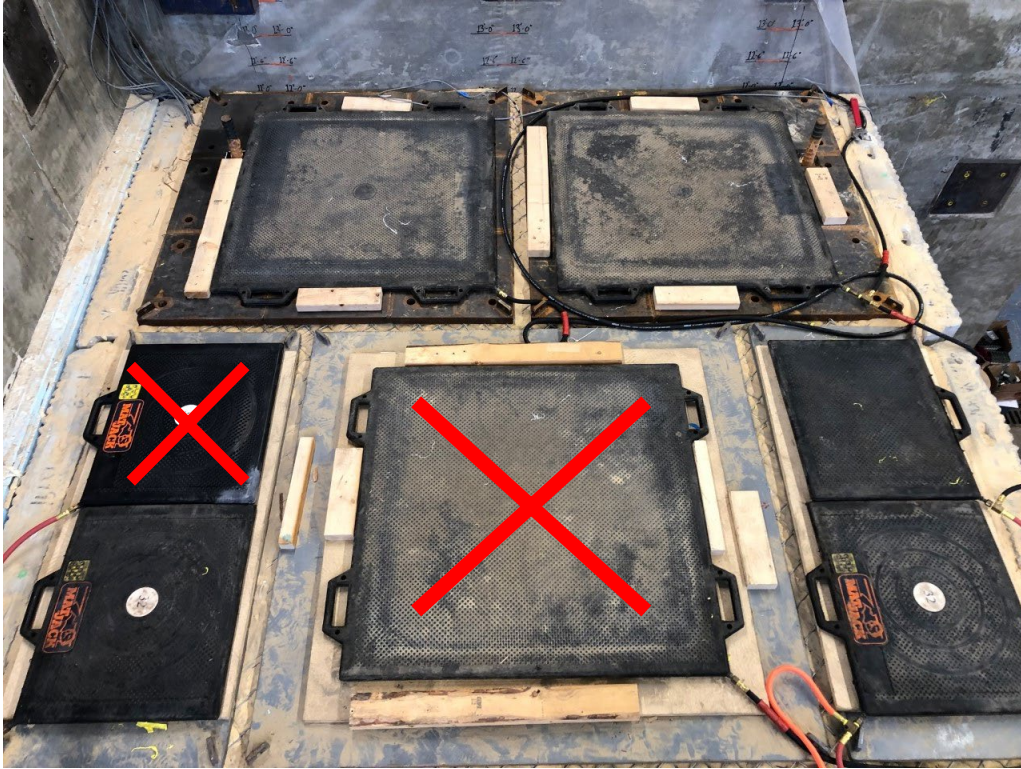
Figure 6-2. Matjack failures on the 103% side during simulated surcharge Phases 1, 2, and 3.
