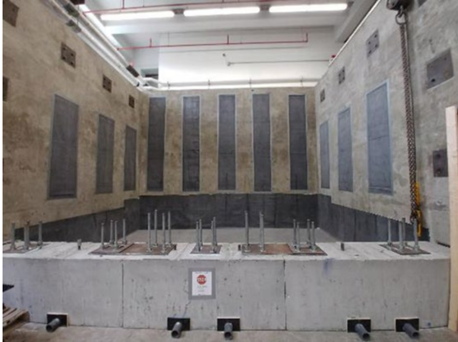
Figure 4-2. Retaining blocks mechanically fastened to strong floor.
