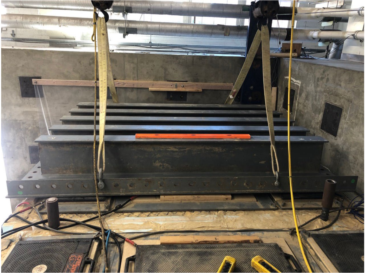
Figure 4-37. First soil box wall in place, resting on matjack system.
