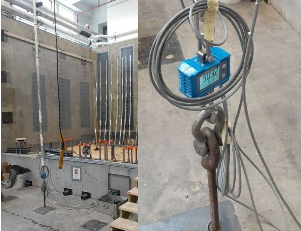
Figure 4-44. Load testing reinforcement strips to develop individual calibration curves.
