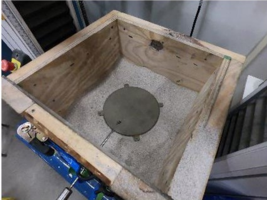
Figure 4-41. EPC test box for calibration after splicing was completed.
