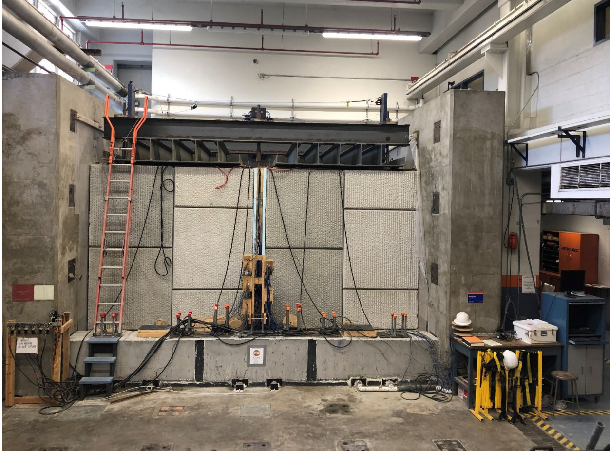
Figure 4-39. MSE wall with reaction frame in place.
