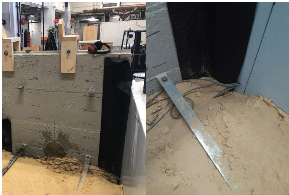
Figure 4-25. Running instrumentation cables through the divider wall.
