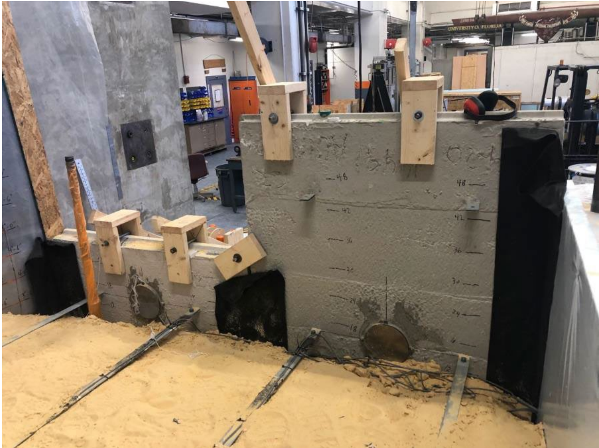
Figure 4-24. Front MSE wall with fatback EPCs mounted to measure horizontal earth pressure.
