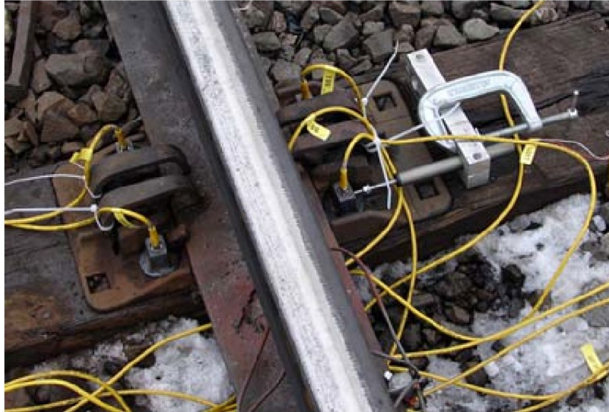
Figure 10. Dick et. al.'s instrumented spike field setup [10]
