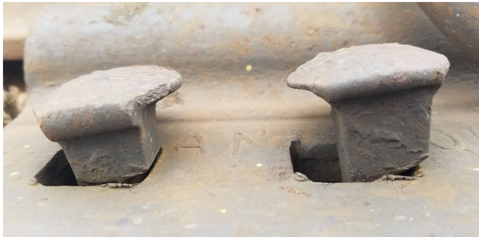
Figure 31. Wear of plate into cut spikes in the longitudinal direction in Pandrol plates
