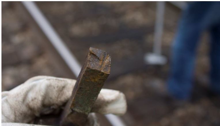
Figure 25. Common spike fracture pattern
