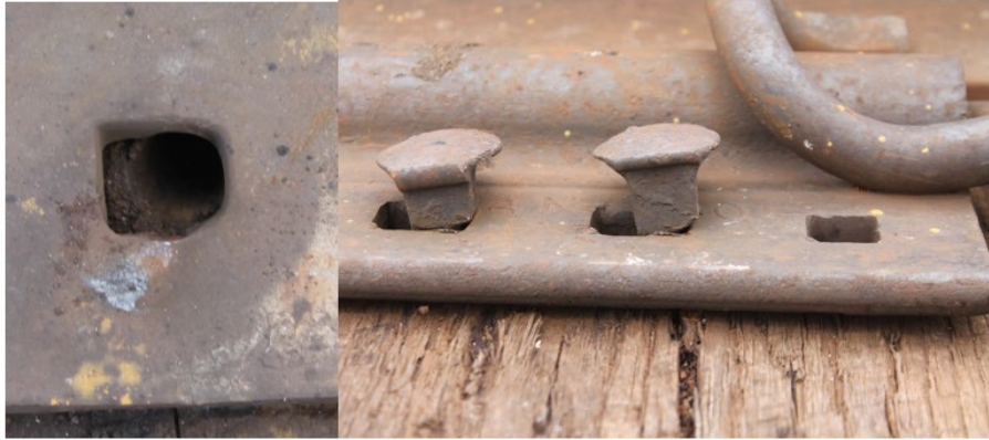
Figure 55. Left: A Victor plate spike hole showing significant wear in the longitudinal direction. Right: Longitudinal plate movement allowed by spike neck wear
