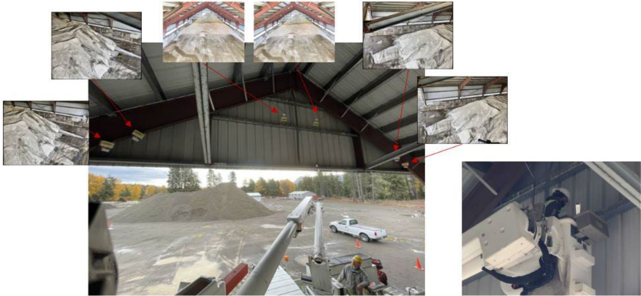
Figure 6.3. Bullfrog facility with three camera pairs at the loading end of the shed.
