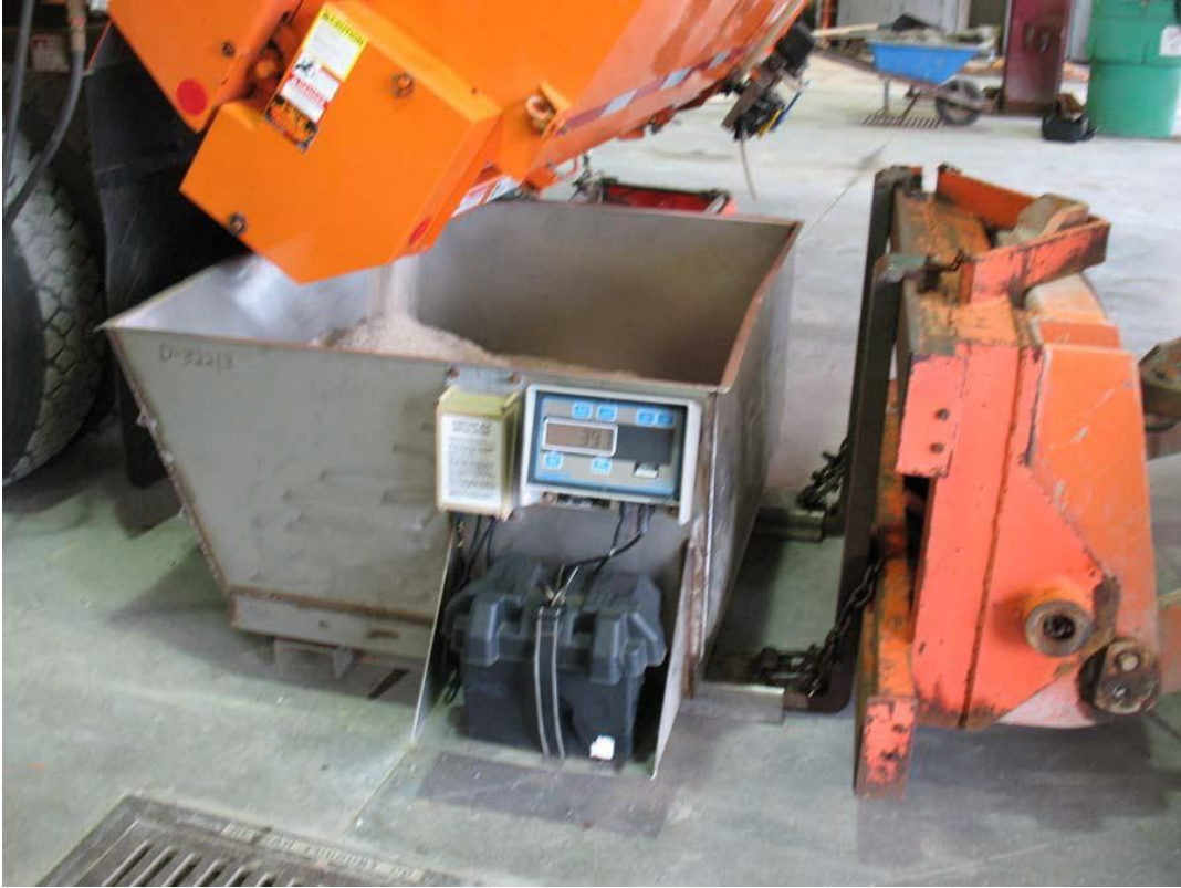
Figure 4. Run material through the system to make sure material is flowing freely and the auger is full
