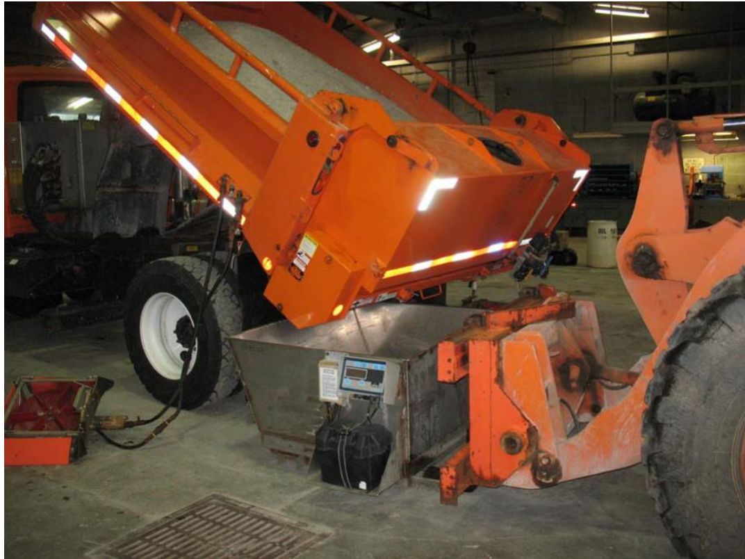
Figure 3. Raising the dump body but make sure the truck or anything else touches the scale
