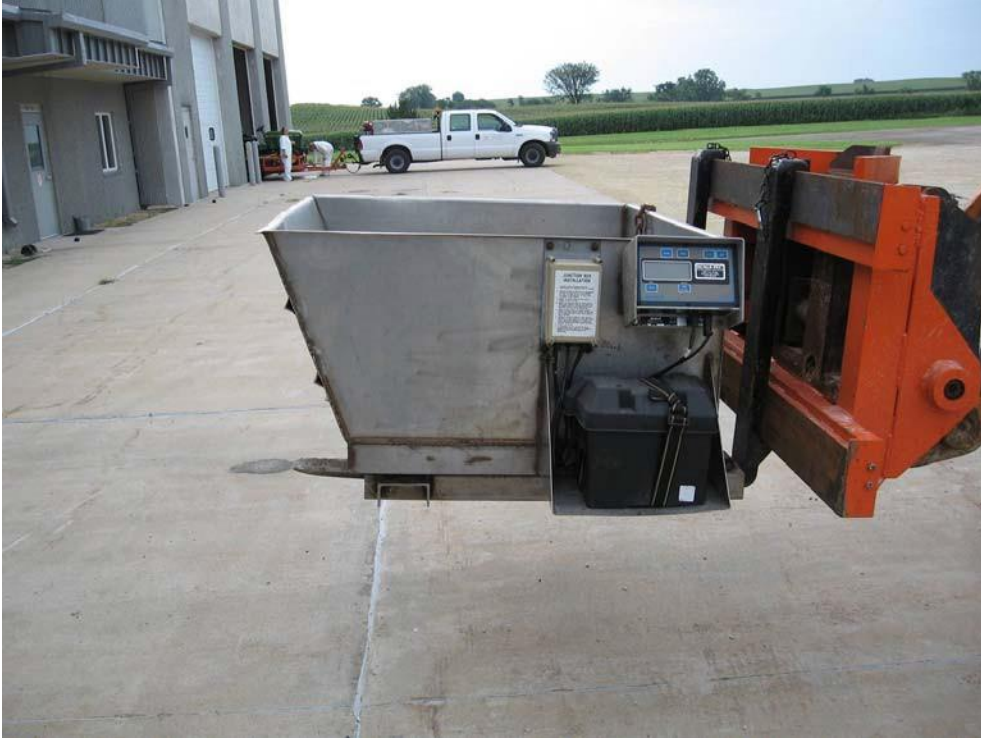
Figure 11. Make sure the battery is properly secured before dumping the salt back into the pile
