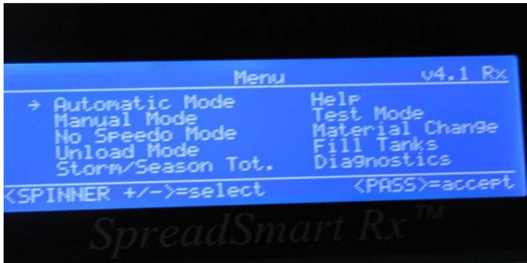
Figure 8. This is the SpreadSmart method to enter data- Check the spreader controller manual on how to enter the calibration number
