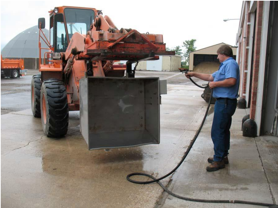
Figure 13. Make sure to wash the scale before putting it away
