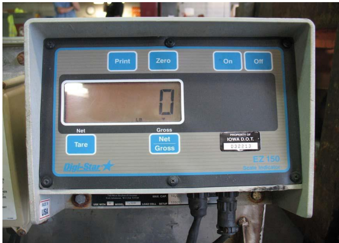
Figure 2. Press the Zero and Net/Gross button to reset the scale
