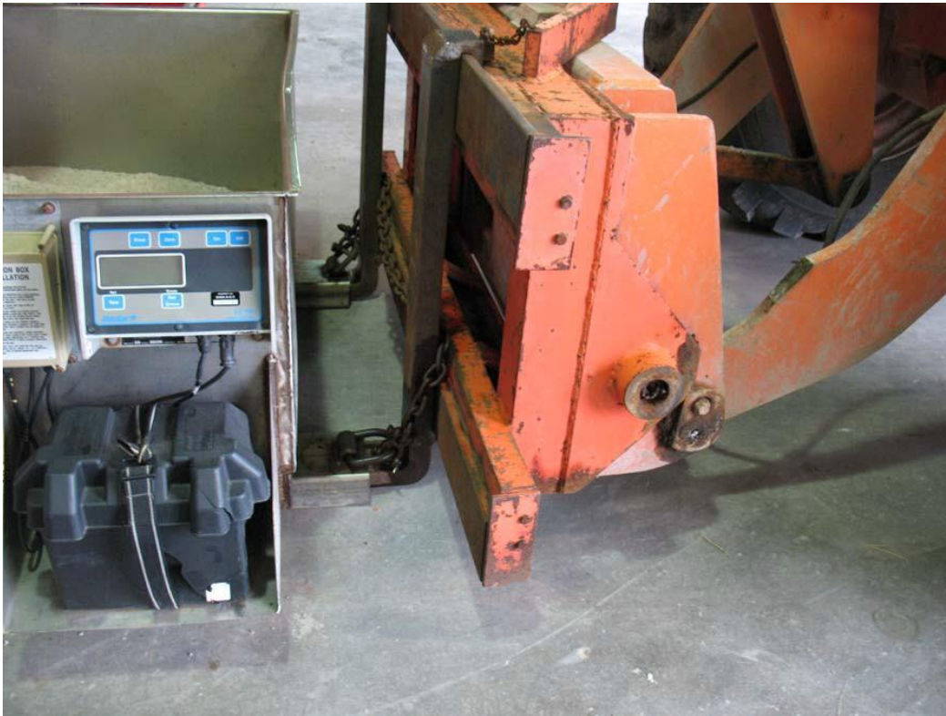
Figure 10. Make sure the scale is turned off and secured to the end loader before dumping the salt back into the pile
