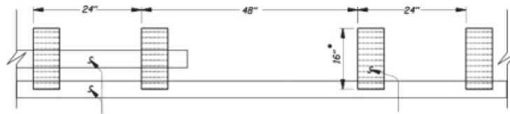
Figure 2.3: Rumble strips (Oregon DOT)
