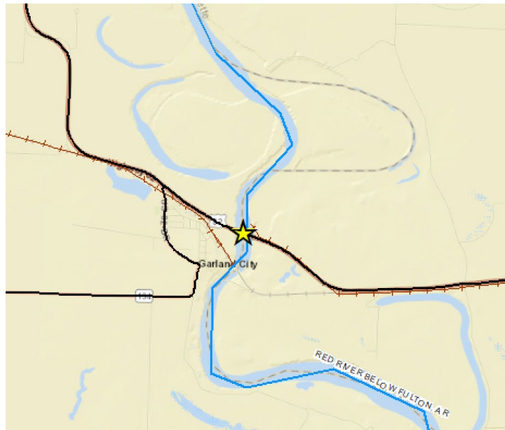
Figure 6: Example of an intermodal node location with all three modes of transportation converging.
