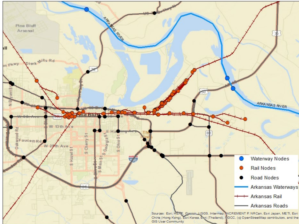
Figure 12: Example of three transportation modes in one area with links and nodes identified from the raw GIS data.
