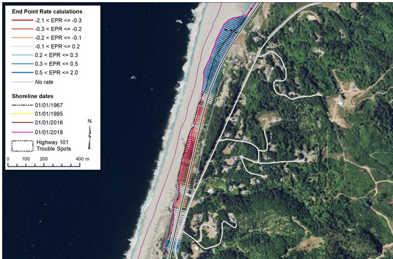
Figure 4.5: Example of change rates determined for transect sites near Ophir Creek on the Southern Oregon Coast in Curry County.
