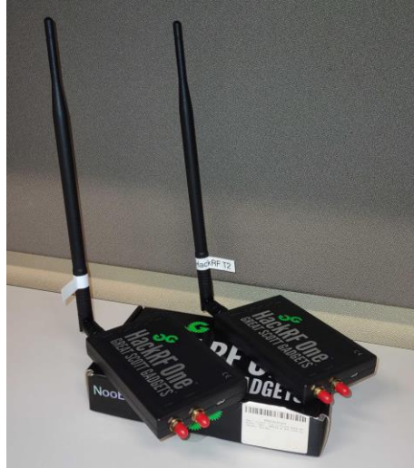
Figure 3.10: HackRF SDR used for BLE experience
