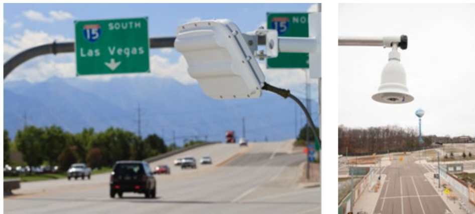
Figure 2.3 [Left] Radar detection sensor and [Right] a GridSmart camera sensor
