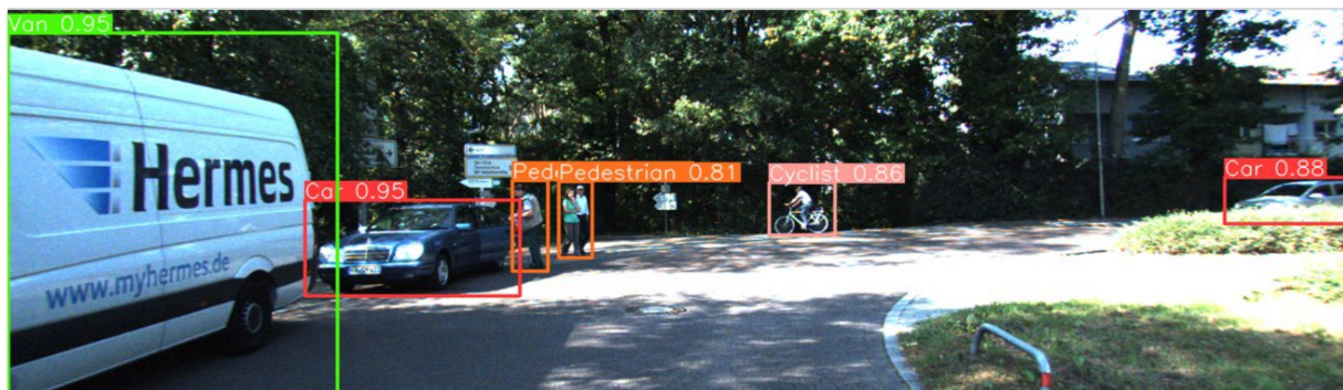
Figure 4.12 An example of the YOLOv5 architecture applied to an image from the KITTI dataset. Each object in the image is assigned a location (box), as well as a probability associated with the classification.
