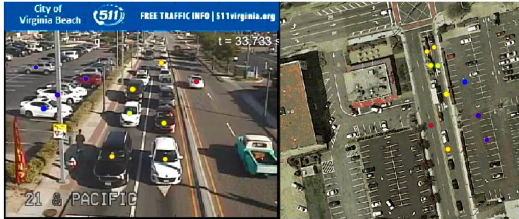
Figure 11. Example output of the Pixel to GPS algorithm. (a) Left side shows traffic camera feed with each detected object. (b) Right side shows map corresponding to the GPS location of each object. 3
