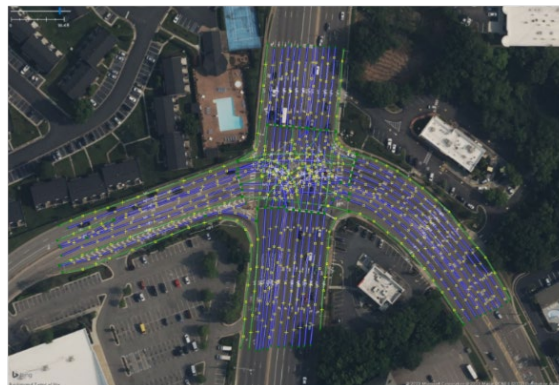
Figure 7. Aerial photo. Lanelets created for one of the risky intersections in Virginia Beach.
