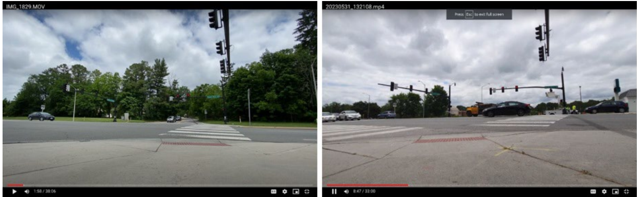
Figure 27. Photos. Two mobile phones placed on diagonally opposite corners of the street such that they capture data from two of the traffic signals.
