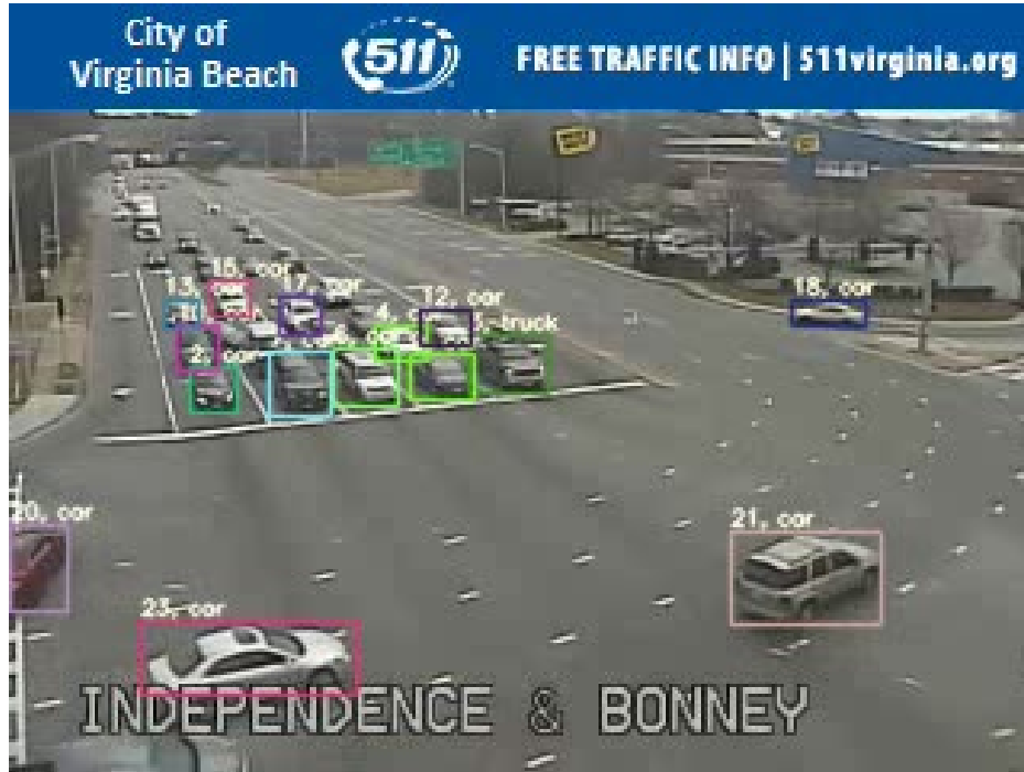
Figure 13. Video image. Sample result on a VDOT video demonstrating object detection with YOLOv7 [54], followed by tracking using BoT-SORT [55].
