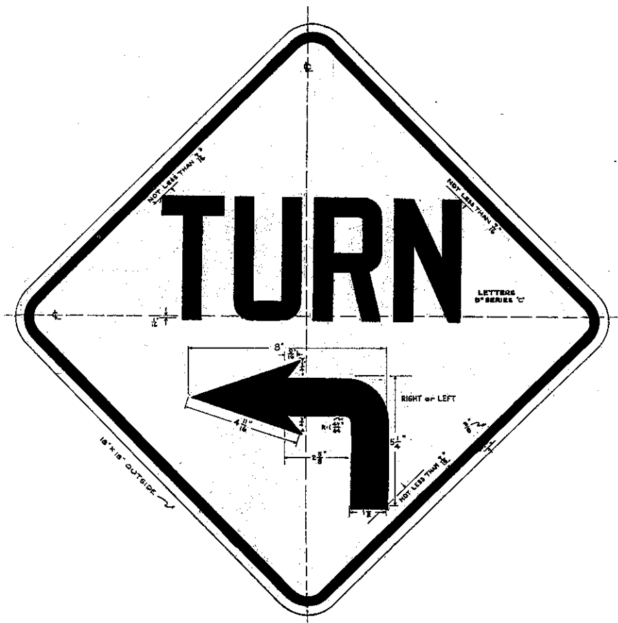
Figure 6: Slow Sign—Traffic Turn Letters, border and symbols, solid black Background, federal yellow (See Recommendation 22)
