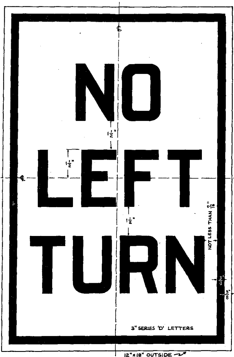
Figure 10: Information Sign—No Turn Letters and border, solid black Background, white
