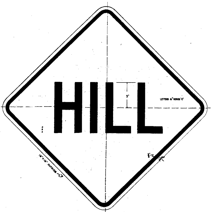
Figure 4: Slow Sign—Hill Letters and border, solid black Background, federal yellow (See Recommendation 20)
