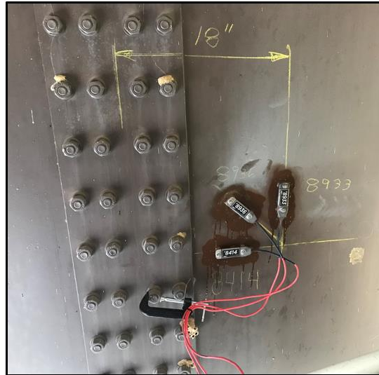
Figure 3-6. Shear Strain Measurement
