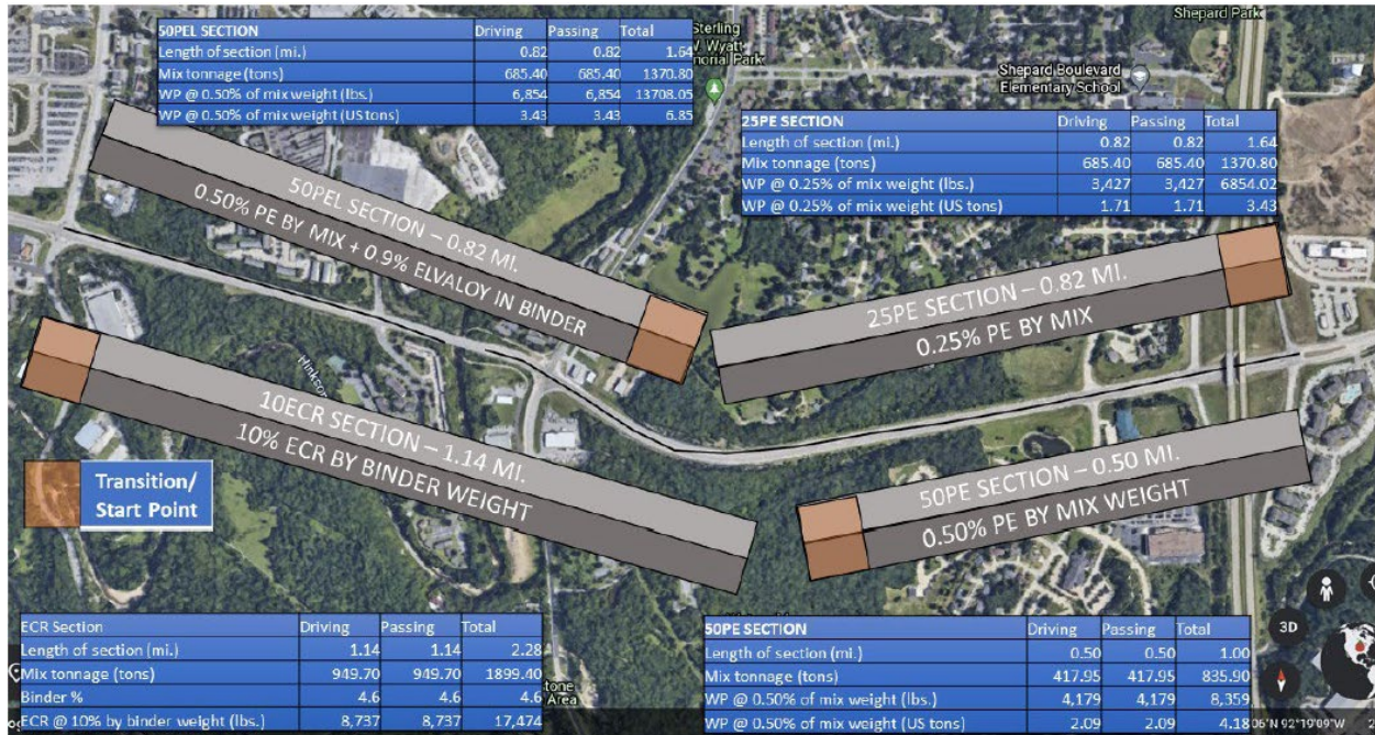
Figure 3.1 Demonstration project layout (Rath et al. 2022)
