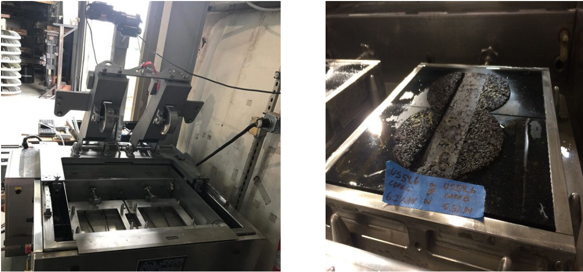
Figure 3-2 Hamburg Wheel Tracking Device: a) Test device b) Mixtures after test
