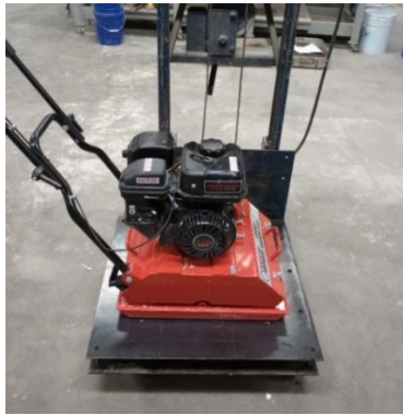
(c) Slab compaction using a vibratory compactor
