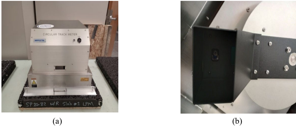
Figure 5-3 The CT meter shown (a) on a fabricated slab and (b) from a bottom view
