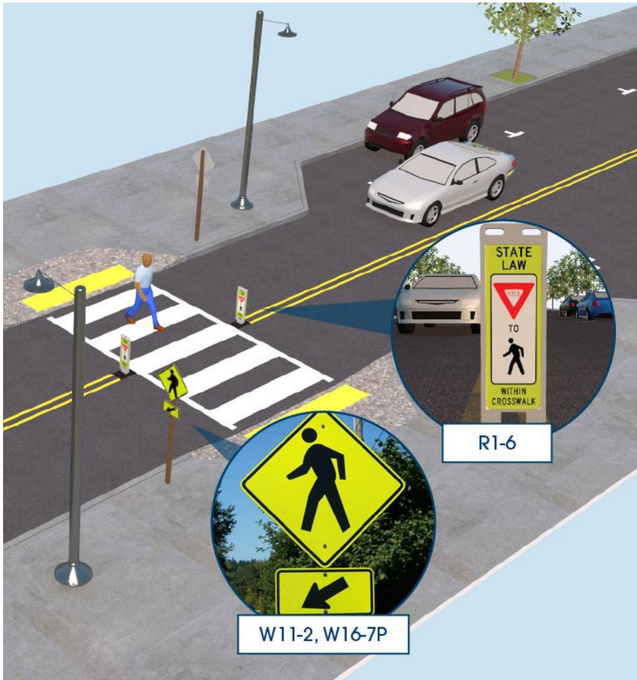
Figure 7-5 Diagram of a High Visibility Crosswalk (Source: FHWA-SA-21-049)
