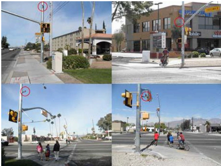
Figure 7-6 Examples of Automated VRU Detection (Source: PEDSAFE)
