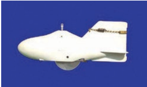
(a) US BM-60 Sampler, 32 lbs 175cc sample size
