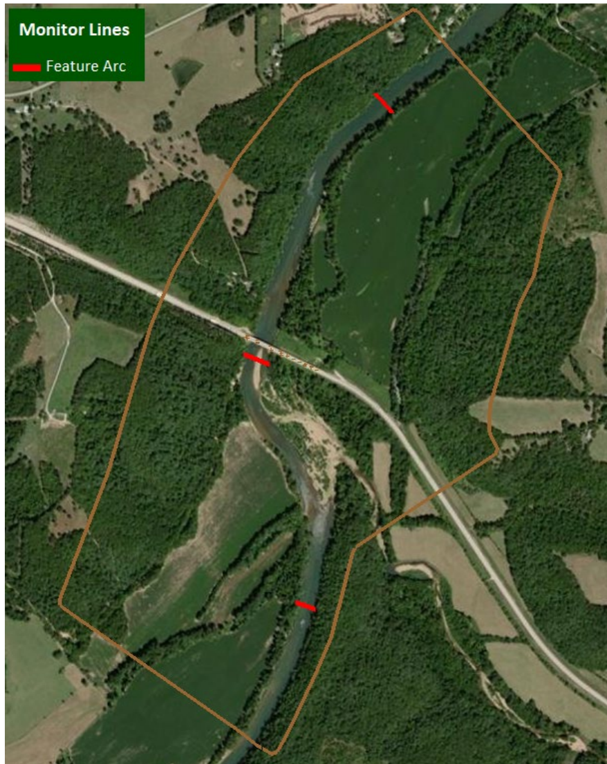
Figure 5-7. Monitor lines used to determine steady-state conditions for the Gasconade River (A-3760) SRH-2D simulations.
