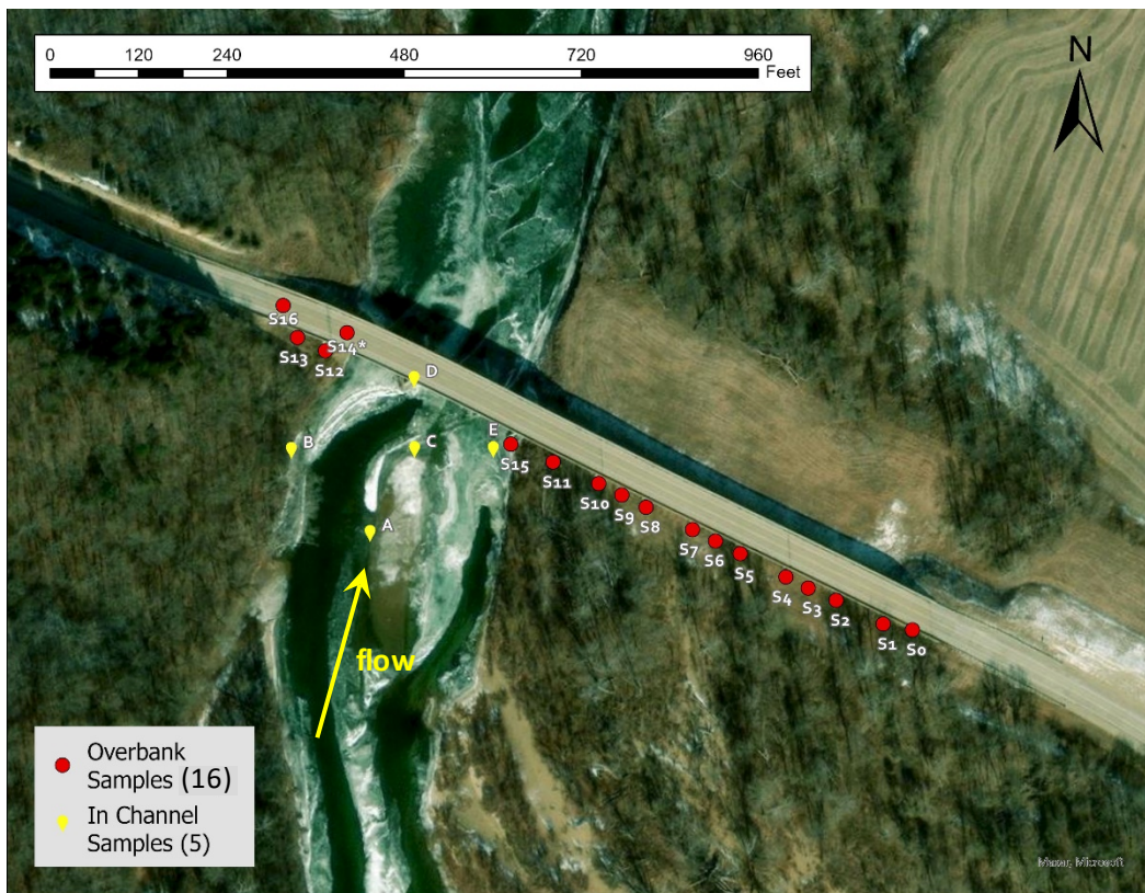
Figure 6-1. Soil sampling locations for the Gasconade River (A-3760) site.
