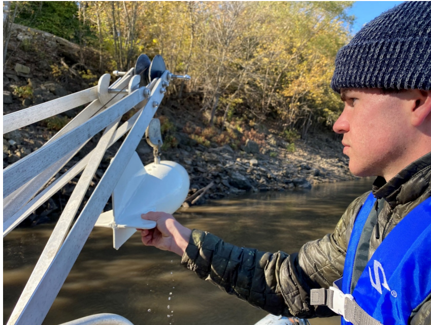
(c) BM-54 sampler being used from a USGS boat using a crane-mounted winch.
