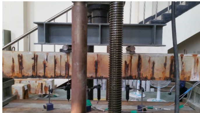
Figure 48 Rust stains indicating corrosion of steel reinforcement in concrete substrate (Jung, Jeong, and Lee 2022)
