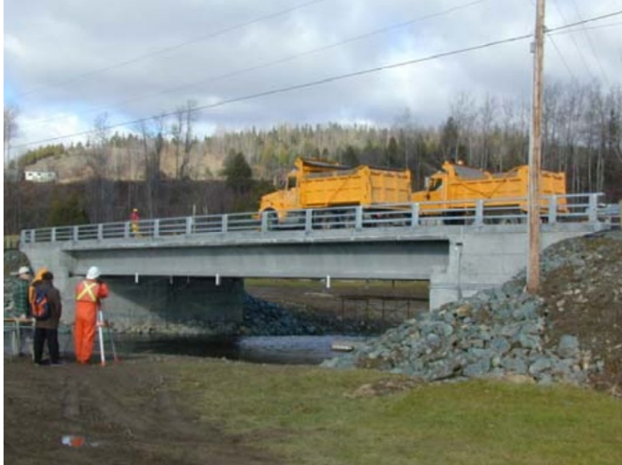
Figure 53 Deflection measurement (El-Salakawy, Kassem, and Benmokrane 2002)
