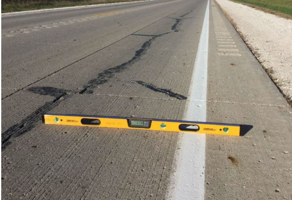
Figure 11 – Sac IA 175 UBOL Left Shoulder Crossslope 1.13%
