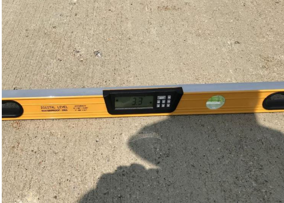
Figure 38 – Shoulder slope 3.3%, Paved 4%
