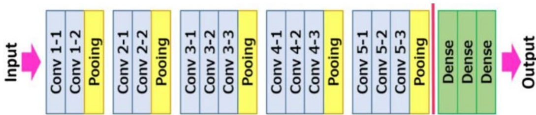
Figure 3.12 VGG16 Architecture (Top 4 Pretrained Models, n.d.)
