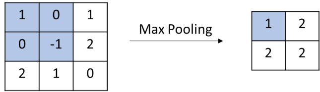
Figure 3.10 Max Pooling Operation
