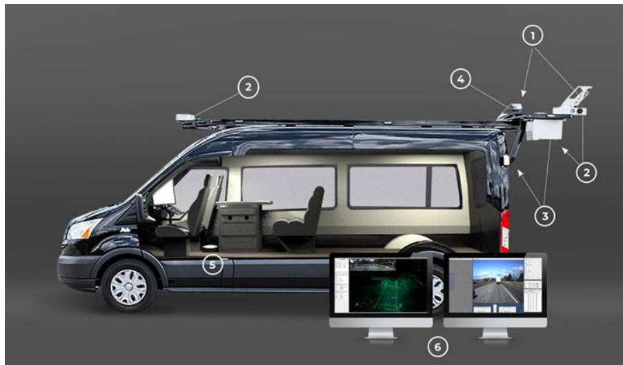
Figure 4.1 Mandli Vehicle Used for Data Collection
