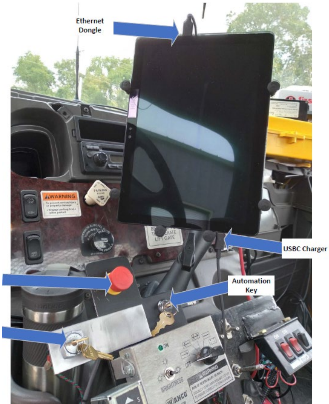
Image 6: Automation keys and Emergency Stop
