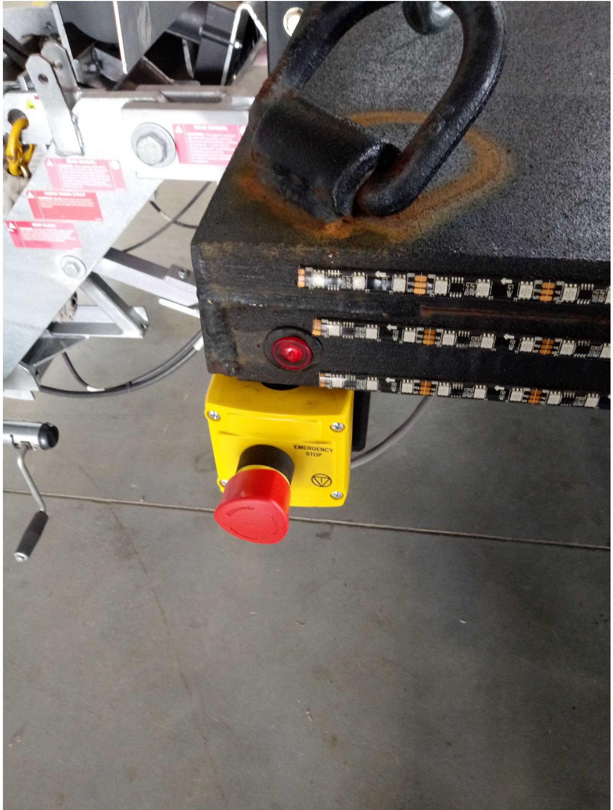
Image 8: One of Four ESTOPS on the bed
