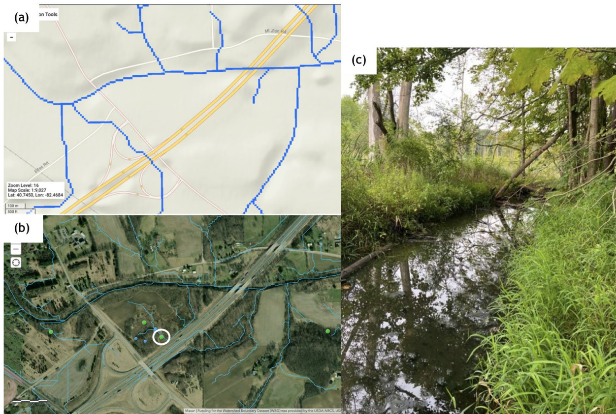
Figure 5. Comparison of extracted channels with streams delineated by the USGS Stream Stats online tool near an interchange at Interstate 70 and State Highway 39 east of Mansfield, Ohio, in the Mohican watershed. (a) Output from streamstats.usgs.gov for streams at this location. (b) Extracted stream channels and field sample points. (c) Existing channel at circled sample point in 5b.
