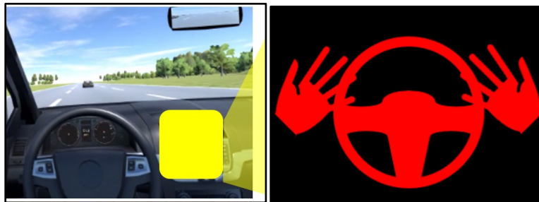
Figure 4. Screen shot (left) and graphic (right). TOR graphic presented in the center console display.
