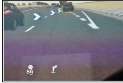
Figure 1. Photo. HMI design using world-relative HUD graphics (i.e., yellow marker that follows the vehicle ahead) and screen-relative HUD graphics (i.e., vehicle speed and navigation directions) [8].
