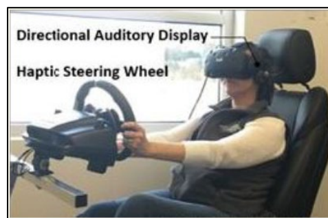
Figure 2. Photo. Picture of driving simulator apparatus with labeled takeover modality features.
