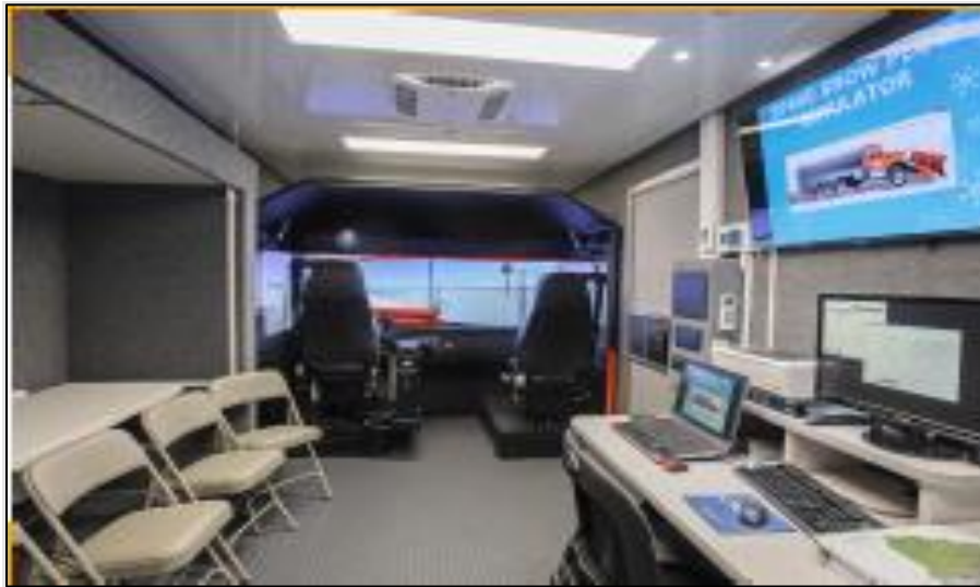
Figure 4. Control Room in Trailer with Instructor Workstation
