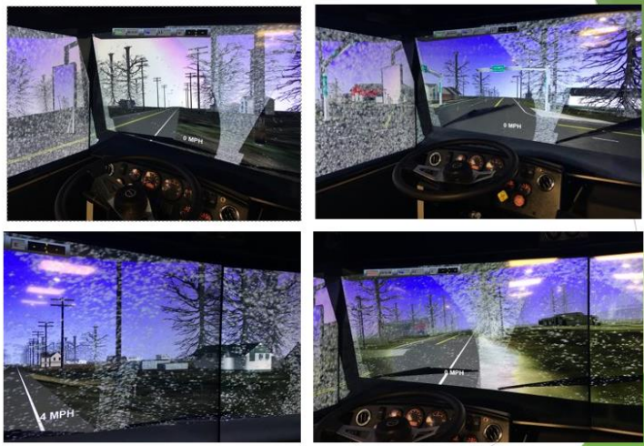
Figure 21. If Vehicle Deviates from Training Route, Collisions may not be Detected
