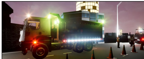
Figure 21. Light Scattering and Bloom of Reflective Ribbon on Construction Vehicle
