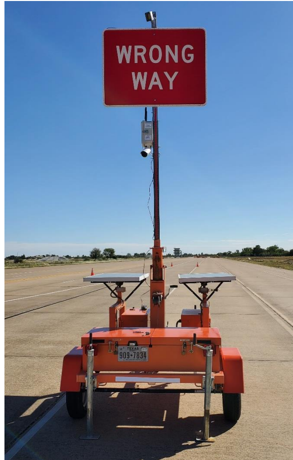
Figure 60. TrafficCalm® Radar 4 with Camera and Controller.
