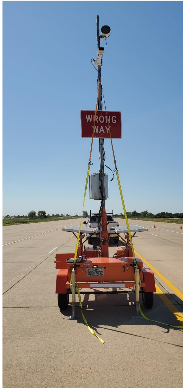
Figure 17. Carmanah® Equipment on Portable Trailer.
