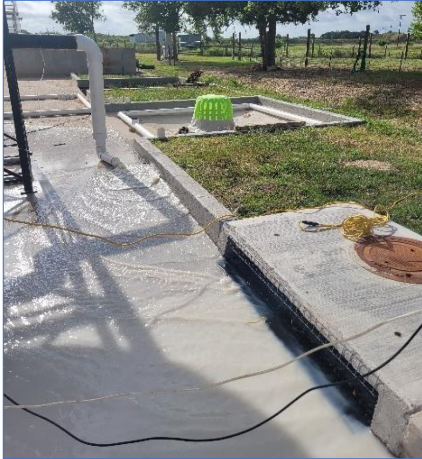
Figure 6. Curb/Gutter Protection Evaluation Test System.
