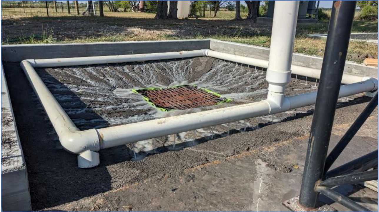
Figure 8. Soil Surface Drop Inlet Evaluation Test System.
