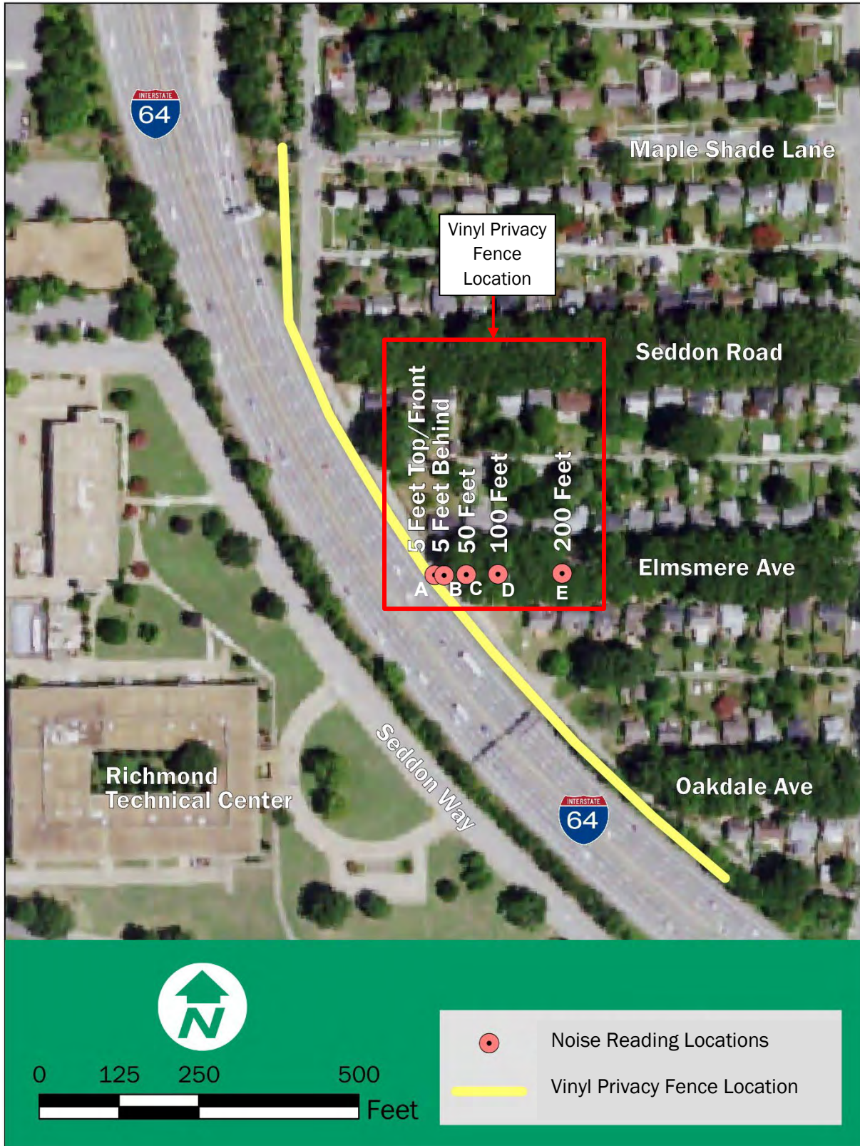
Exhibit 1: Richmond, Virginia Noise Measurement Locations
