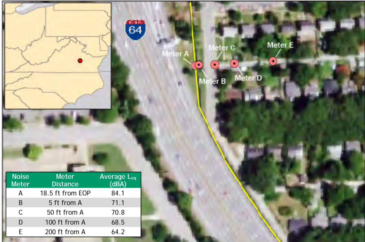
Figure 4.4: Richmond, Virginia Vinyl Privacy Fence & Concrete Noise Wall Average Noise Dropoff
