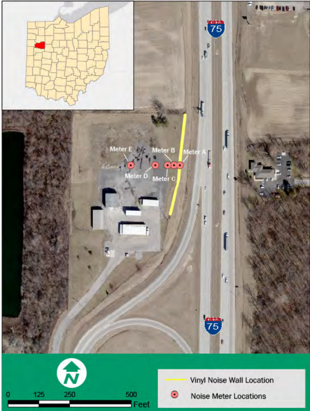
Figure 3.15: Lima, Ohio New Vinyl Noise Wall Post-Construction NMP Map
