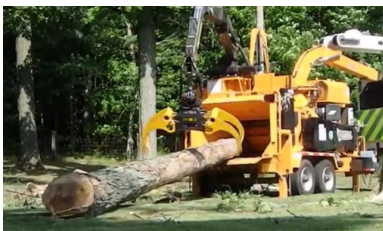
Bandit 2090 whole tree chipper with Kesla Loader
