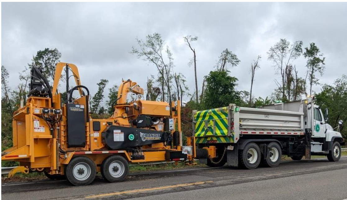
Photo 5: Bandit 2090 chipper attached to a truck with a dump bed in July 2022 operations.
