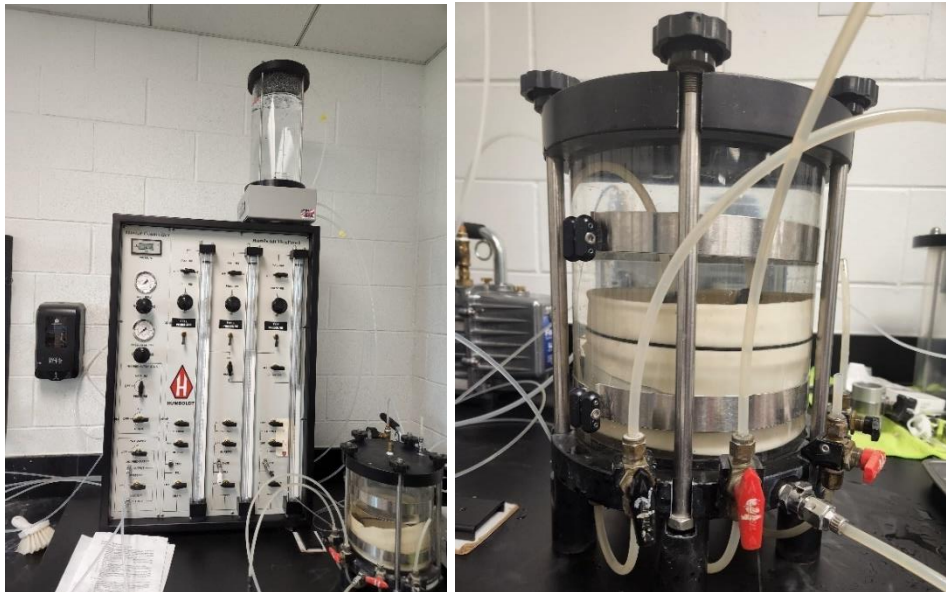
Figure 81. Permeability Test (ASTM D 5084).
