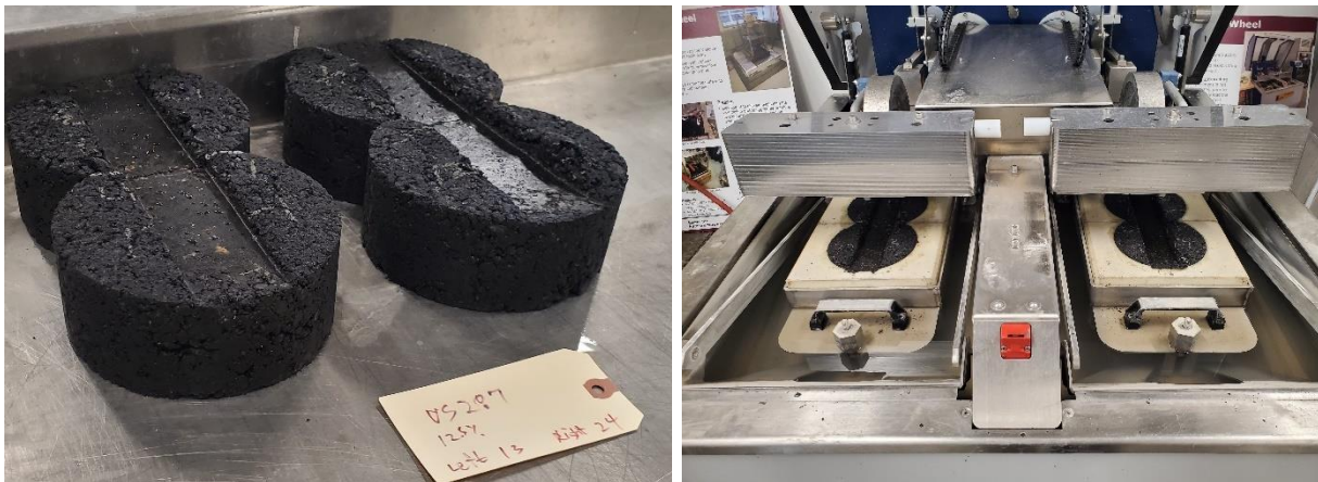
Figure 77. Example Hamburg Test (Tex-242-F).
