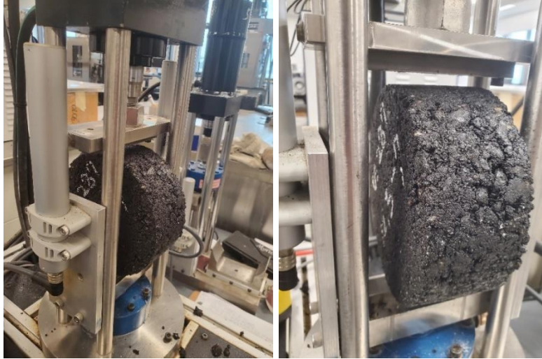
Figure 79. Example IDEAL-CT Test.
