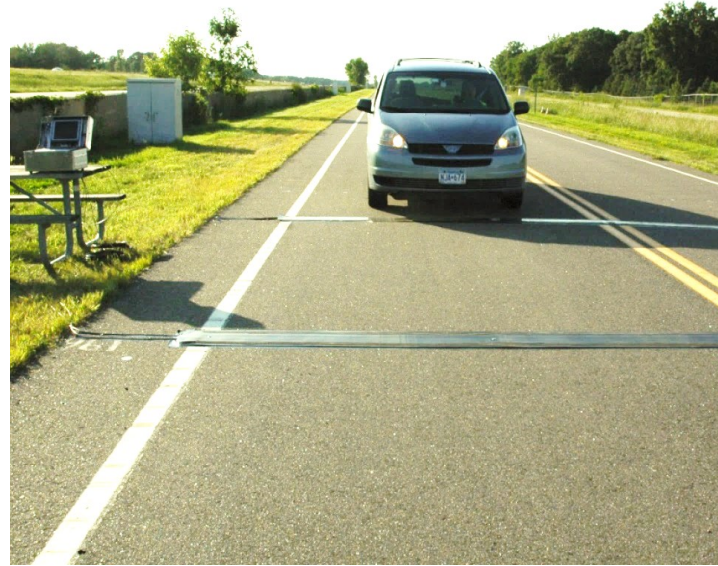
2. Portable Pavement WIM
