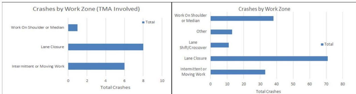
Figure 19 - Crashes by type of Work Zone. Left shows results for Dataset1, where TMA was involved. Right shows results for Dataset2
