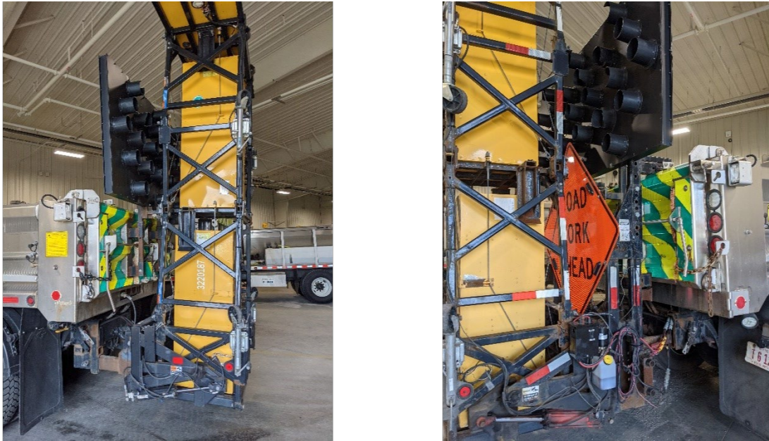
Figure 23 -TMA systems of different kinds installed on dump-trucks
