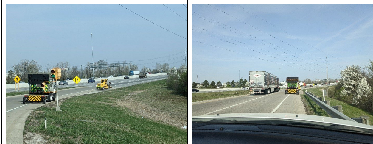
Figure 25 - TTMA in a shoulder sweeping operation on I-270. Left - Operating on a narrow on-ramp, TTMA occupies travel lane restricting flow of traffic. Right - TTMA passed by a tractor-trailer on the left when travelling on the on-ramp. In both situations, the TTMA displayed a caution sign
