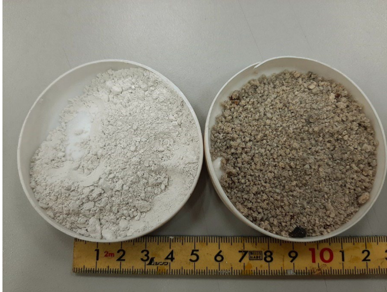
Figure A.5. Granulated Blast Furnace Slag ( Right ) and Ground Granulated Blast Furnace Slag ( Left ) (Dinh 2023).
