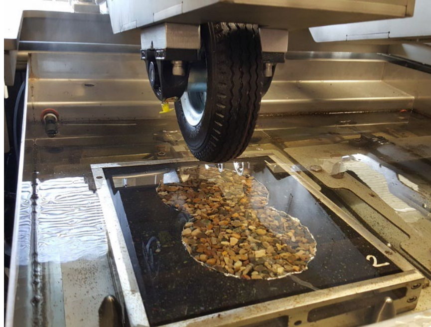
Figure B.4. Hamburg Wheel Tracking Device Retrofitted with a Rubber Wheel.
