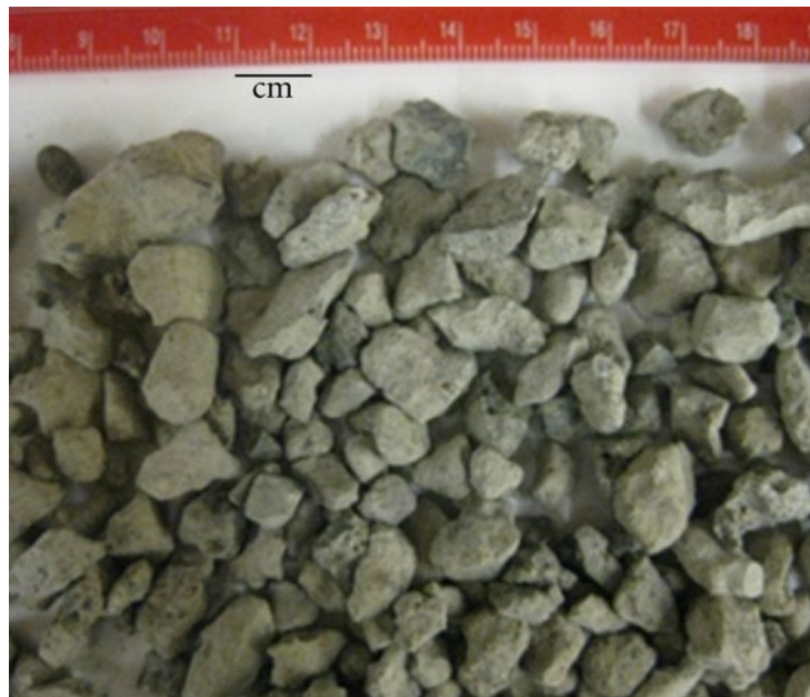
Figure A.8. A Sample of Gravel-Sized Particles of BOF Slag (Yildirim and Prezzi 2011).
