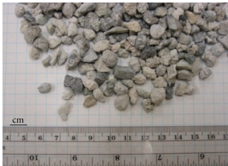
Figure A.9. A Sample of Gravel-Sized Particles of EAF Slag (Yildirim and Prezzi 2011).
