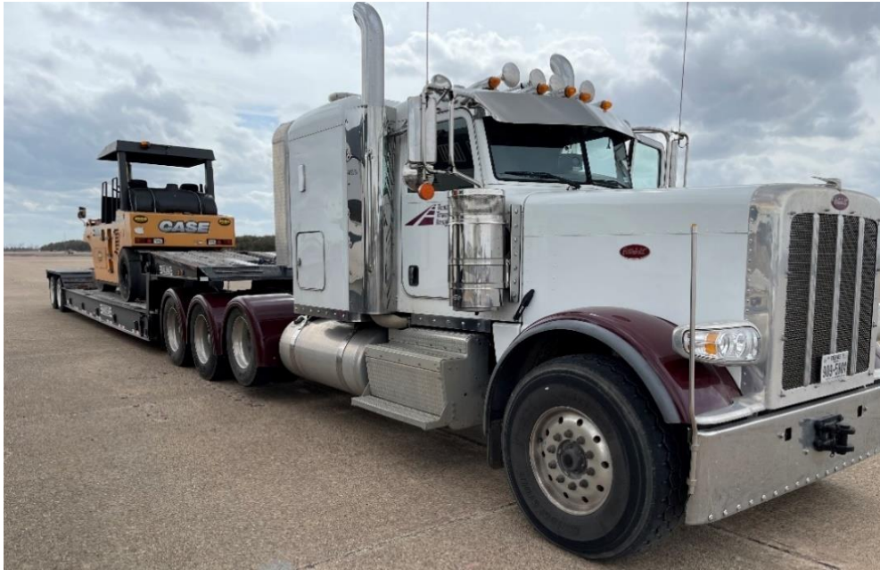
Figure 5.8. TTI Tractor-Trailer Loaded with a Roller Compactor.
