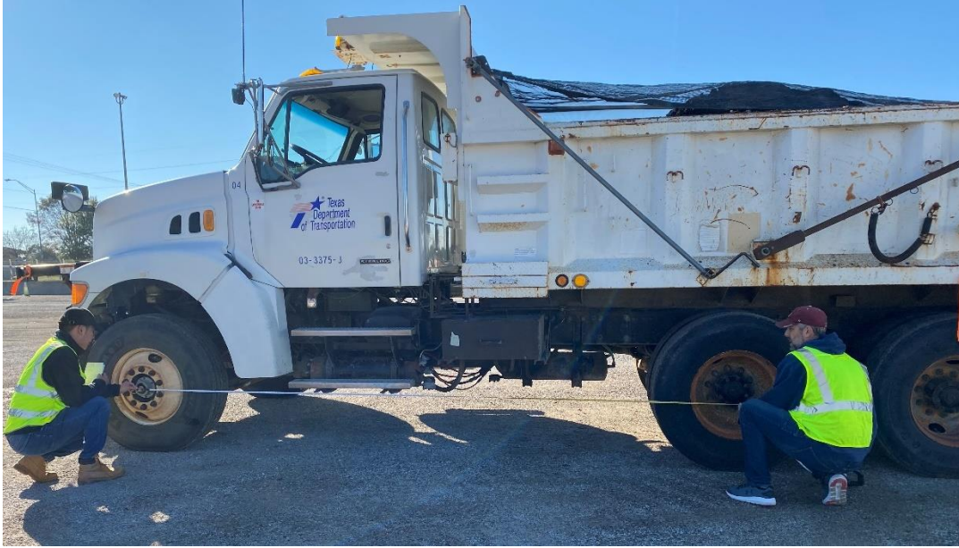
Figure 8.19. Truck Dimension Measurement.
