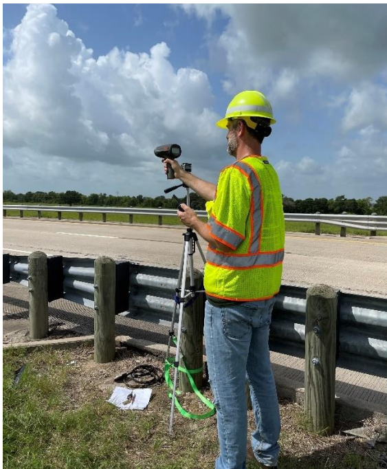
(a) Speed Measurement with a Radar Gun
