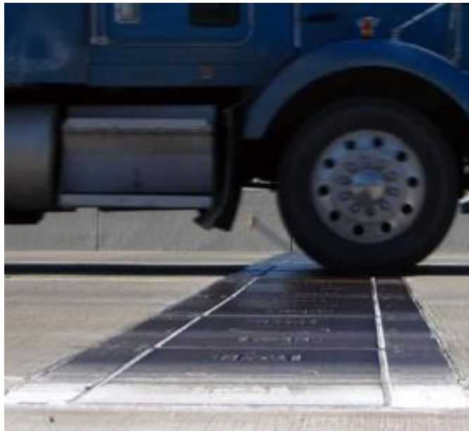
Figure 2.5. Load Cell–Based Weight Sensors (IRD 2019).
