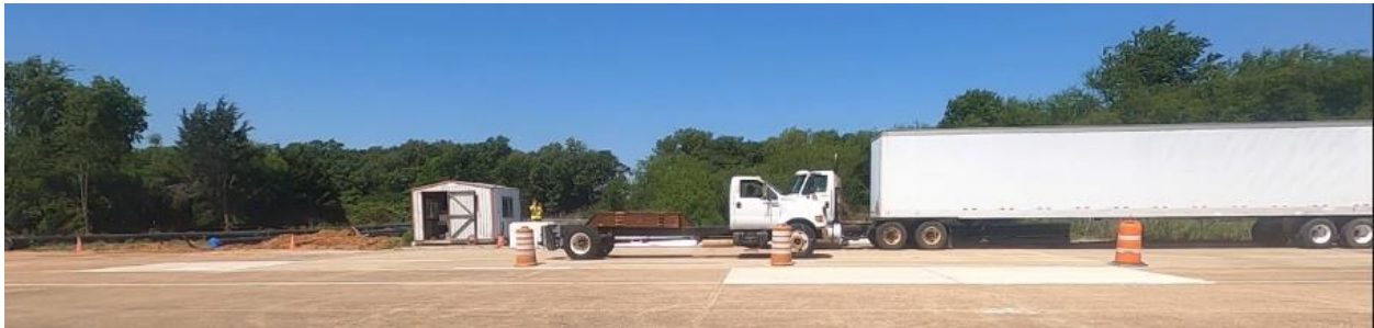
(b) Two Vehicles Reached Midspan of the RELLIS Bridge from Opposite Directions
