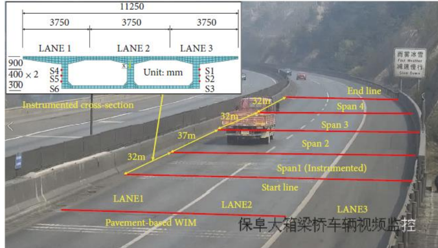
Figure 2.18. Instrumented Section of the Tested Bridge (Jian et al. 2019).
