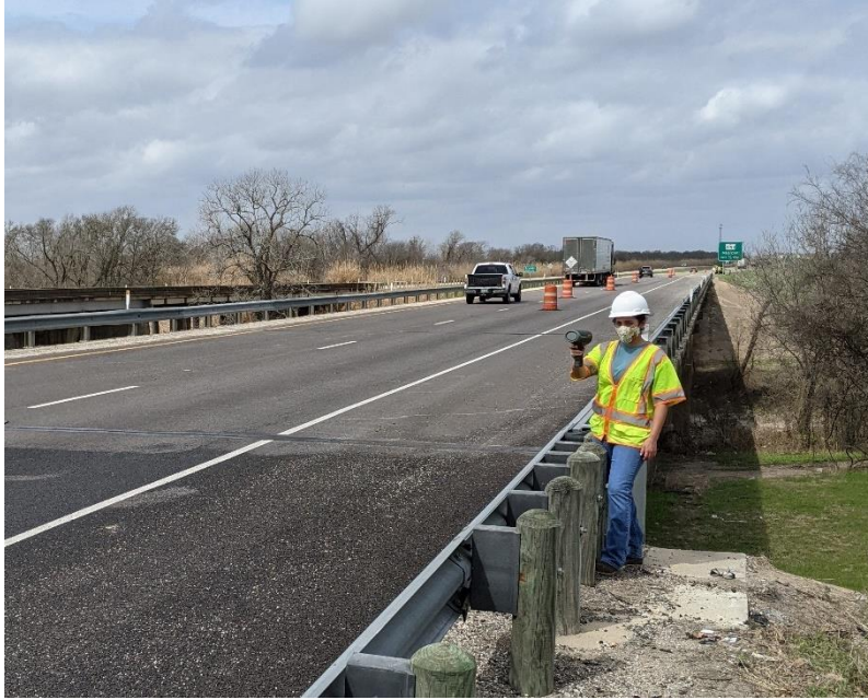
Figure 5.13. Speed Measurement with a Radar Gun.
