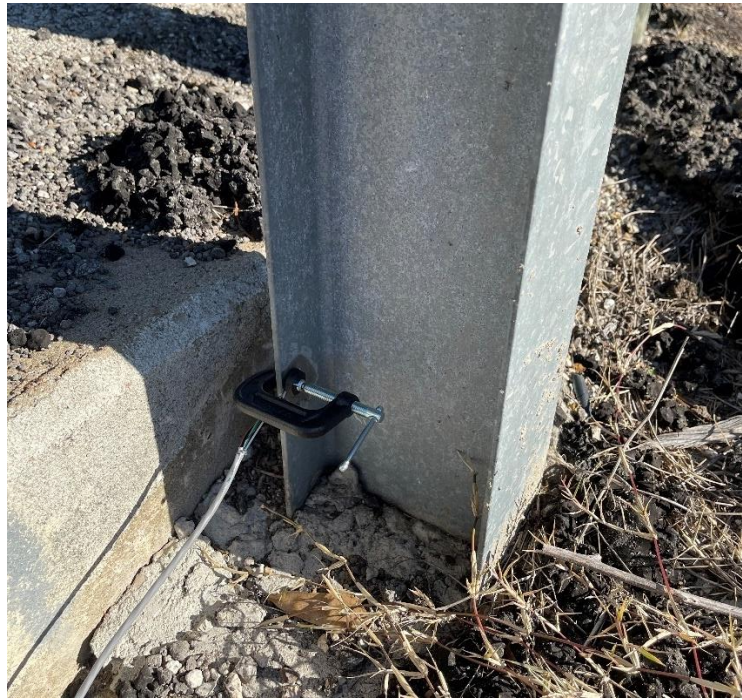
(b) Ground to the Steel Post
