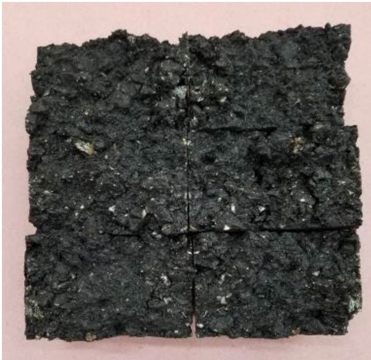
Figure 34 Granite, Gyratory Compaction, Additive B
