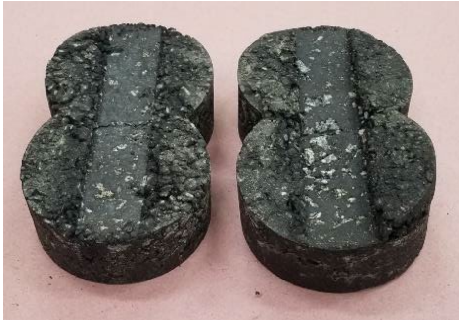
Figure 51 Granite, Lime Additive
