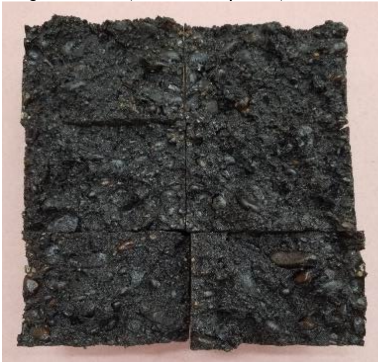
Figure 38 Gravel, Gyratory Compaction, Additive A, Conditioned
