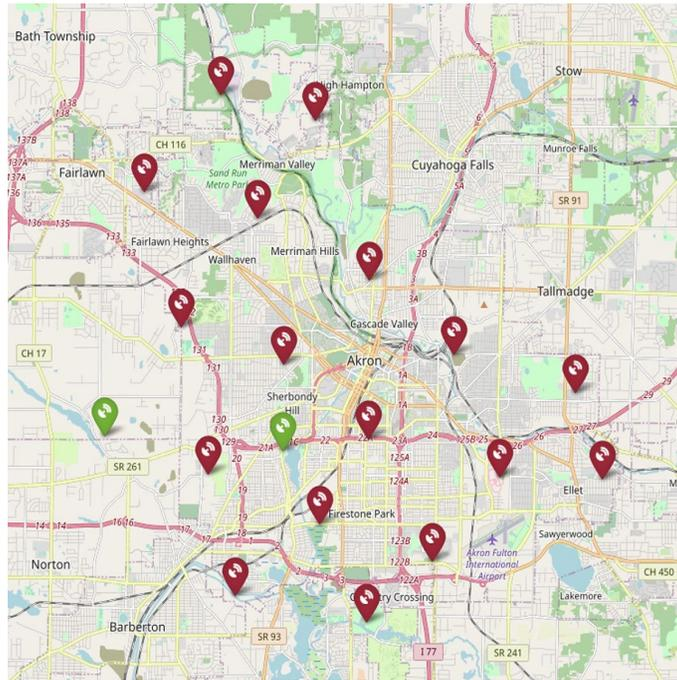
Fig. 10 Optimal locations of mixed sensors in Akron (red markers represent the location of radars, and the green markers the location of acoustic sensors)
