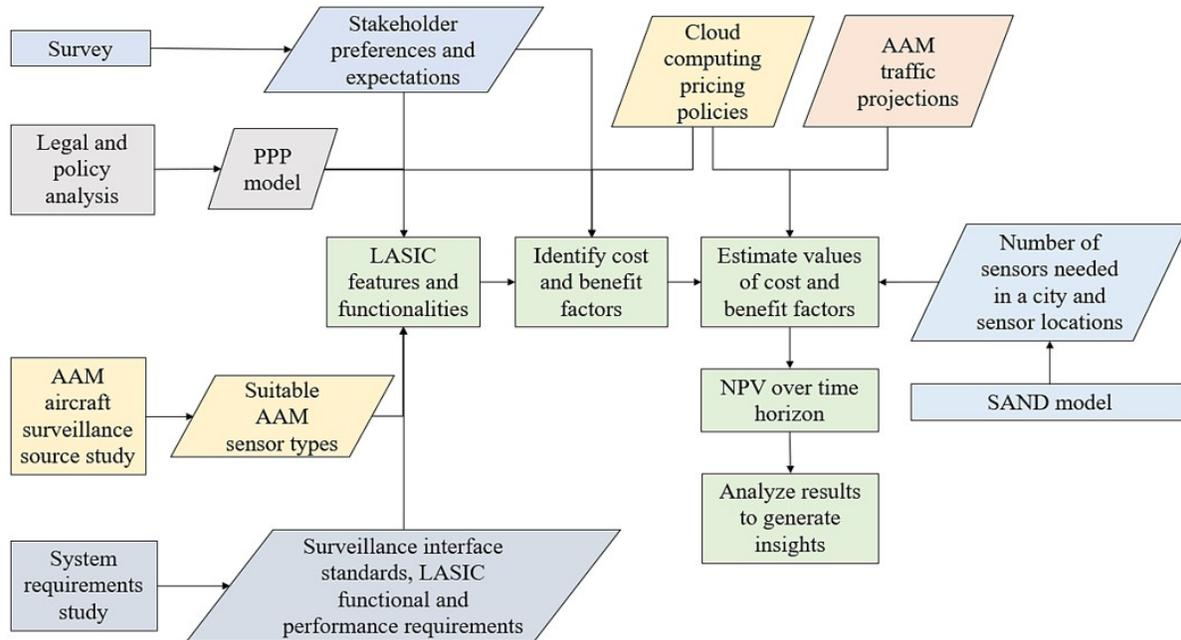
Fig. 2 A flow chart illustrating the steps associated with cost-benefit analysis of LAASS
