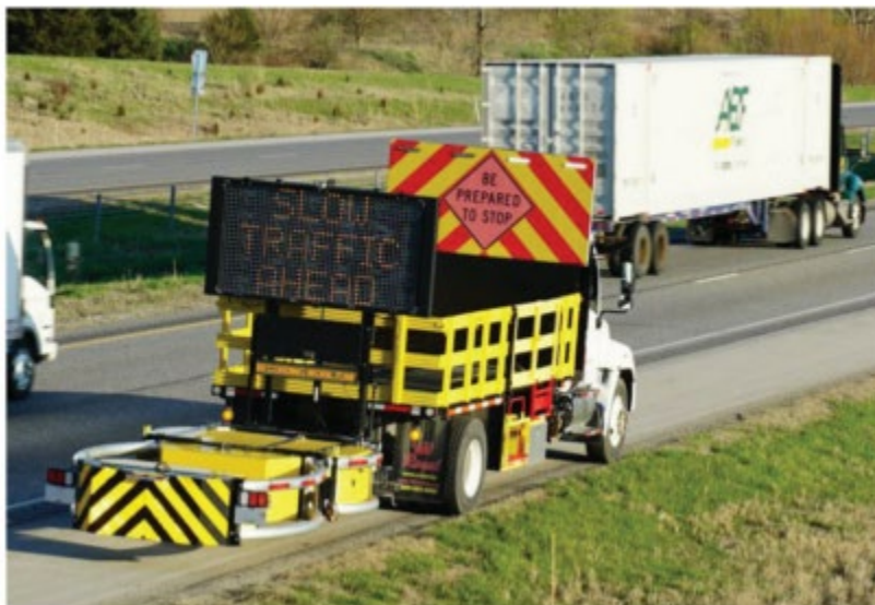
Figure 1. INDOT Queue Truck in a Work Zone.
