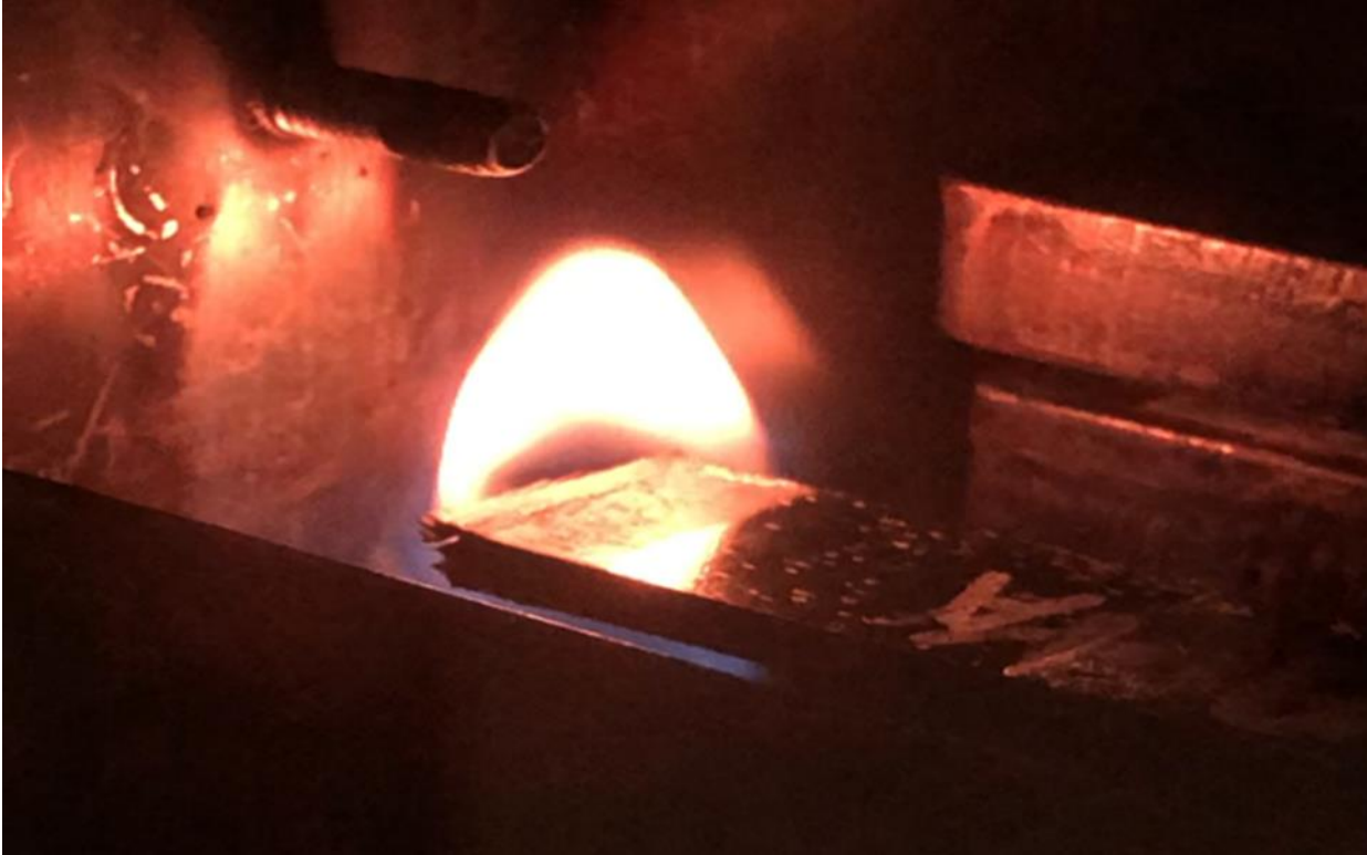
Figure 32. 21-ply cross-ply Cytec UNCO specimen during horizontal burning test with Bunsen burner
