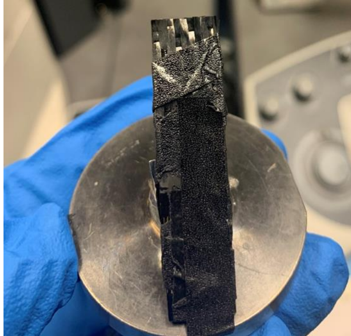
Figure B - 5. Sample preparation: pristine 4-ply cross-ply [0/90/90/0] Hexcel specimens before SEM imaging
