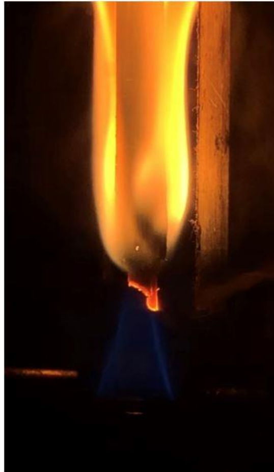
Figure 31. 21-ply cross-ply Cytec UNCO specimen during vertical burning test using Bunsen burner
