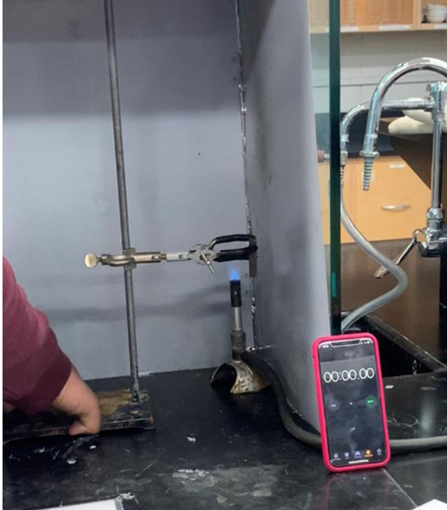
Figure B - 4. Vertical fire test setup of a Hexcel composite specimen
