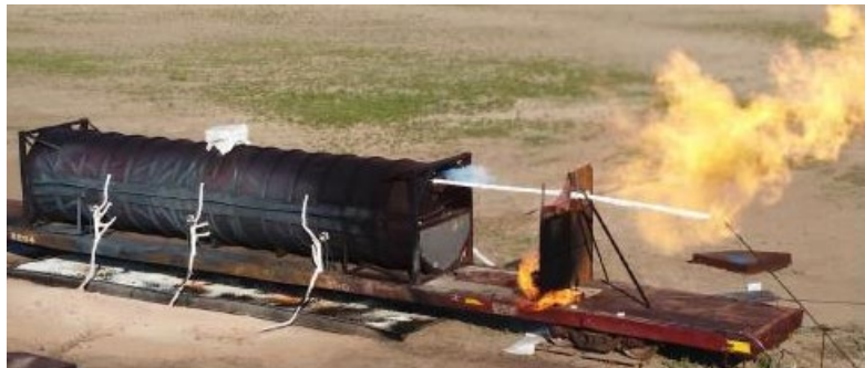
Figure 1. Jet Fire of PRV exhaust during fire test of LNG filled UN-T75 tank (FRA, 2023)
