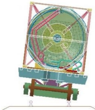
Figure 5. View of model showing LNG within the tank (shown graphically as ‘dots’) at initiation of rollover
