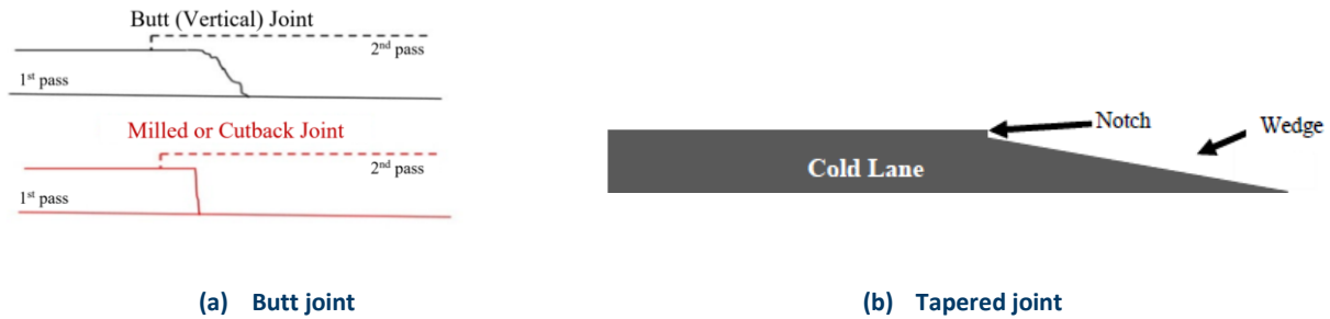
Figure 5.6 Schematic of butt and tapered joints.
