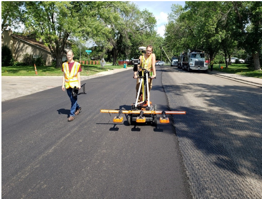
Figure 3.1 DPS data collection on the unconfined joint with a 6 in (150 mm) offset – Xerxes Road #1, MN
