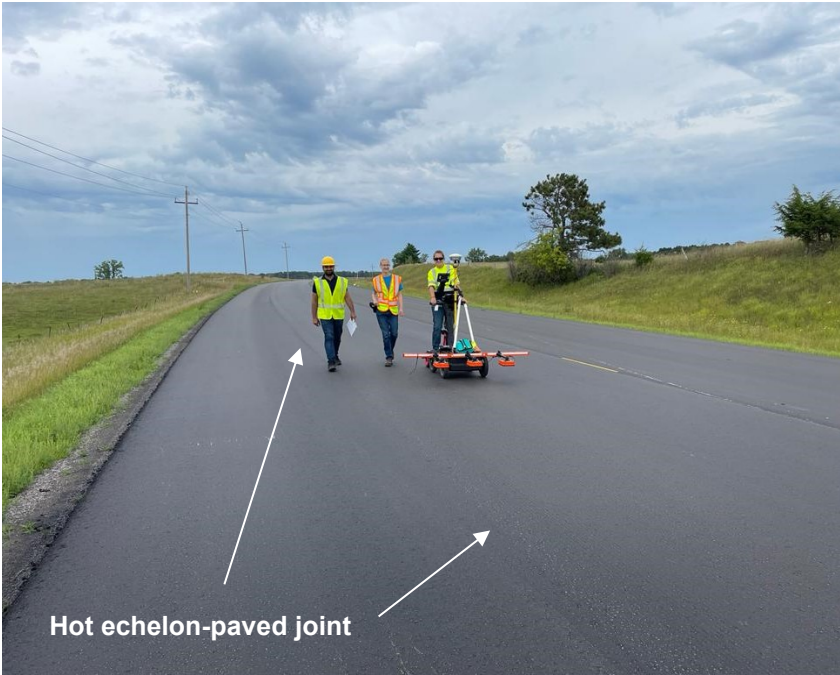
Figure 3.4 DPS data collection on the cold confined, and hot echelon paved joints – Manning Trail, MN
