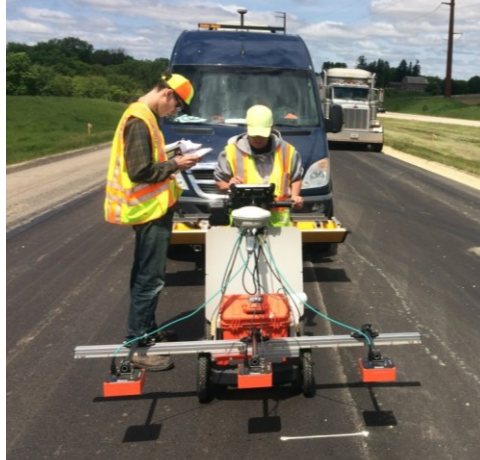
Figure 2.12 Three-sensor Density Profiling System (courtesy of MnDOT)
