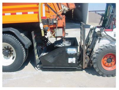
This simple tray for deicing sand, coupled with the new methods developed by MnDOT research for calibrating snowplows, is expected to save at least \$400,000 over three years, for a benefit-cost ratio of 4.5-to-1.
