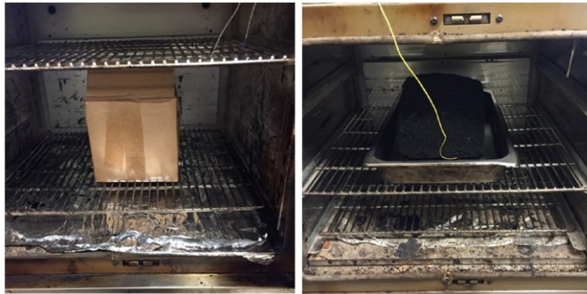
Figure 30. Reheating of Boxed versus Unboxed Loose Mixture Samples (Lemke et al., 2019)
