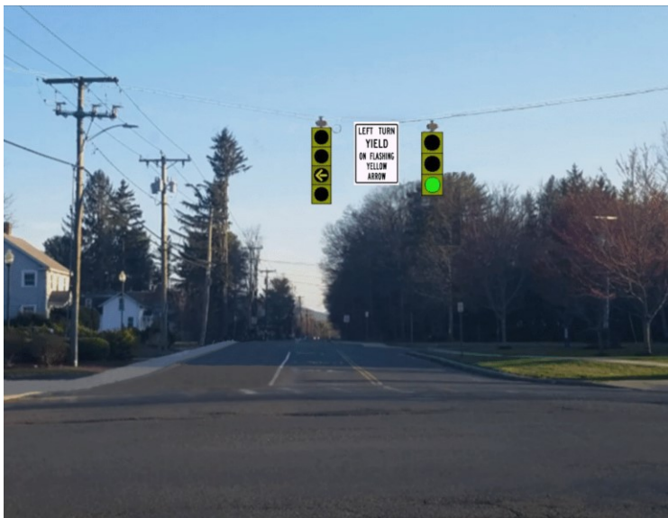
Figure 2.16 Question 10 - Four-Head Flashing Yellow Arrow with Sign. The image was animated to show flashing.
