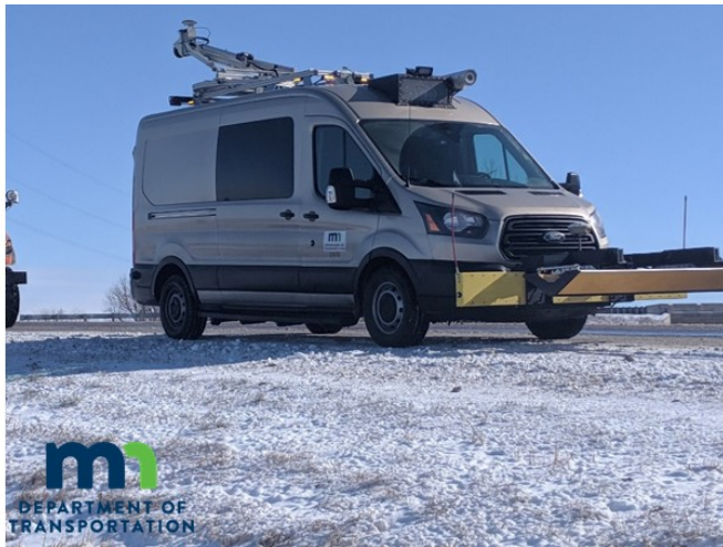
Figure 14-2 Road Doctor Survey Van
