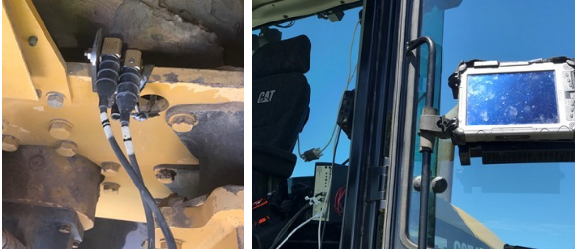
Figure 3-6 UTEP Moduli ICMV Accelerometer (Left) and Onboard Display (Right) (Chang, et al., 2023)
