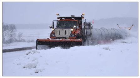
A truck's mass impacts fuel economy. The gradual weight decrease of a snowplow that occurs after unloading anti-icing or deicing material can range from six to 12 tons. In this study, the weights of an empty truck and a truck fully loaded with salt were used to calculate fuel efficiency.
