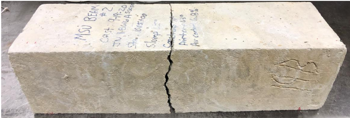
Figure 6-32 Typical beam break – I-196 EB JPCP project
