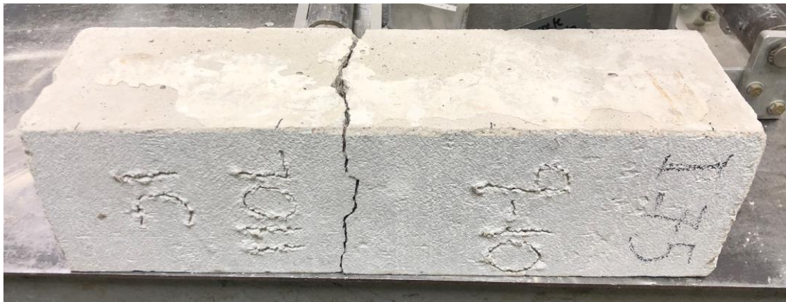
Figure 6-33 Typical beam break – I-75 SB JPCP project
