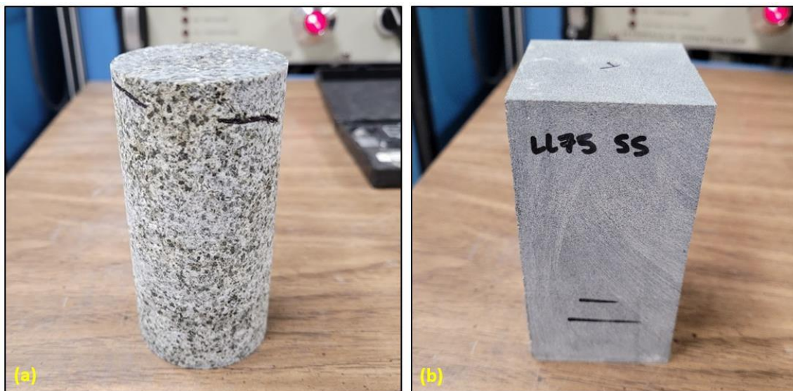
Figure 2.3 Images of (a) cylindrical and (b) prism samples before strength testing. Prominent discontinuities are marked on each sample in black.
